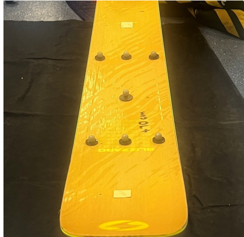
Figure 2.7: Example of one instance of MOCAP marker pattern for roving output impact test.
