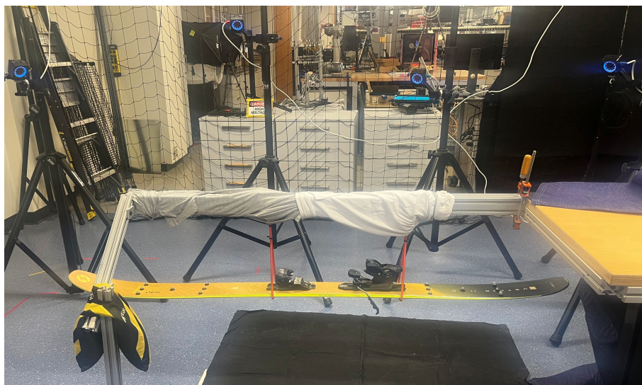
Figure 2.6: Shows overall set up for MOCAP-based roving output impact test; MOCAP, markers, and the same impact hammer from the accelerometer-based tests.
