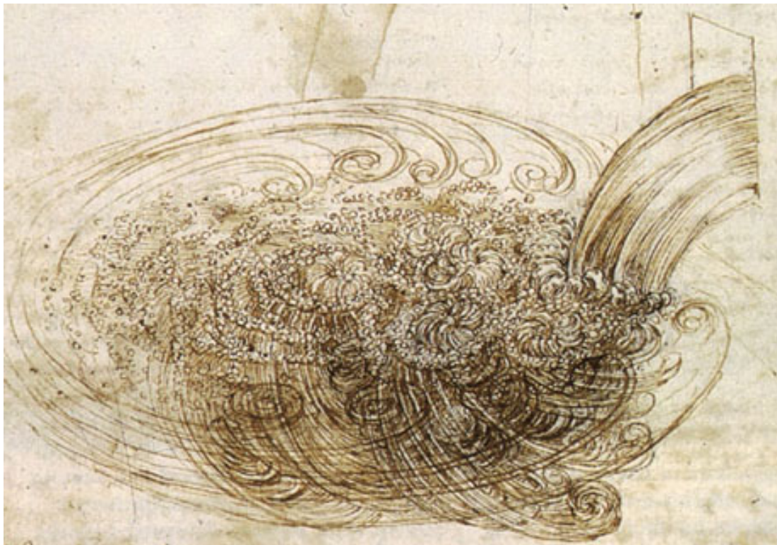
Figure 1.1: Leonardo Da Vinci's illustration of the swirling flow of turbulence. The sketch elucidates that water flowing out of an orifice has eddying motions of different scales ( courtesy: The Royal Collection ©2004, Her Majesty Queen Elizabeth II ).
