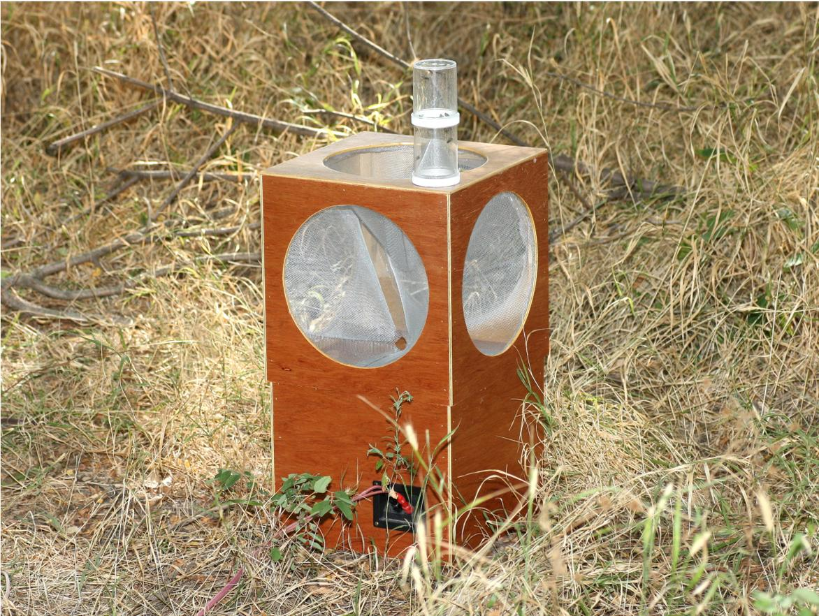
**Figure A.2** The live trap deployed in the field. Captured flies are visible in the holding jar assembly at the top of the trap.
