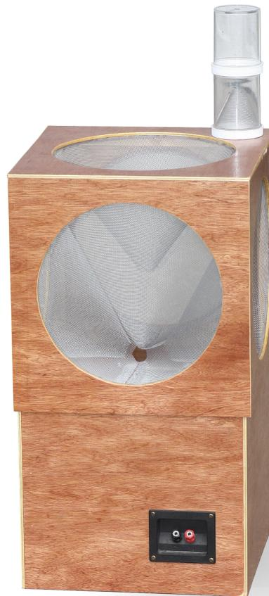
**Figure A.1** The complete trap with the loudspeaker box on the bottom, trapping unit above the loudspeaker box, and holding jar assembly on top.
