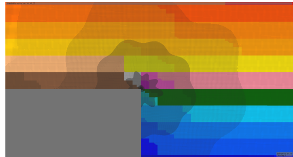
(d) Grid alignment and partition near corner singularity
