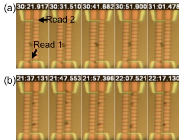
Figure 130: (a) SPB trapped on Read 1 SV, (b) SPB trapped on Read 2 SV.
