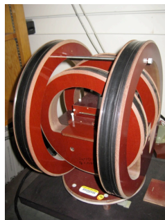
Figure 75: B-H loop tracer for measuring the SV hysteresis curve. The loop tracer consists of a solenoid coil and a pickup coil.
