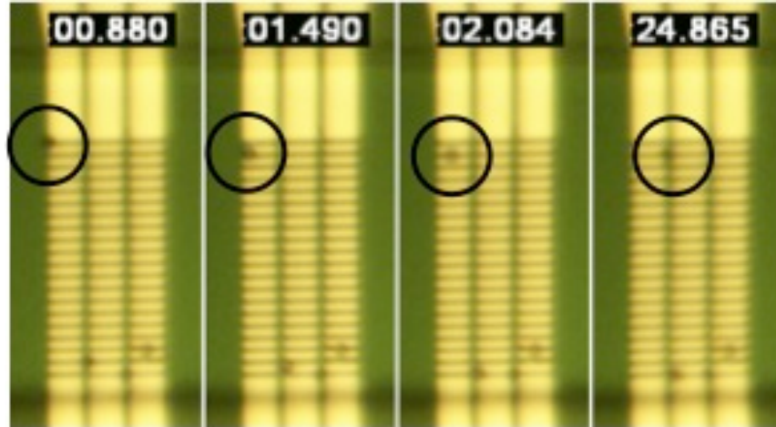
Figure 112: Video stills showing a 2.8 \mu\text{m} SPB released from Write 1 SV and captured by a Write 2 SV.
