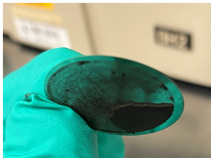
Figure 3.6: A target produced using an over-saturated C_{60} -toluene solution
