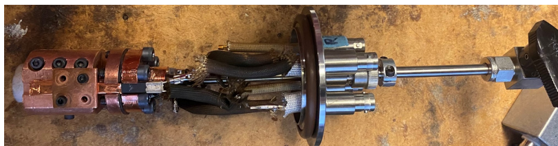
Figure 3.2: The oven used to sublimate C_{60} for PVD.
