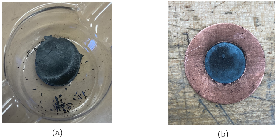
Figure 3.10: (a) A pellet of pure C_{60} created using a hydraulic press with 127,000 psi. (b) A pellet of reused C_{60} from previous front desorption tests on a copper backing plate, made using a hydraulic press with 10,000 psi
