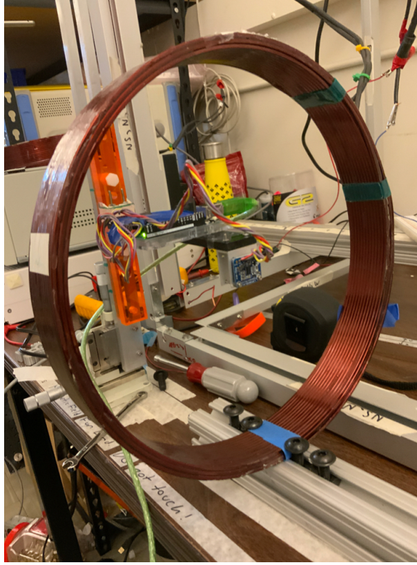
Figure 7.3: One of the setups used to test the gain of the and offsets of the magnetometer using the JILA eEDM generation I coils
