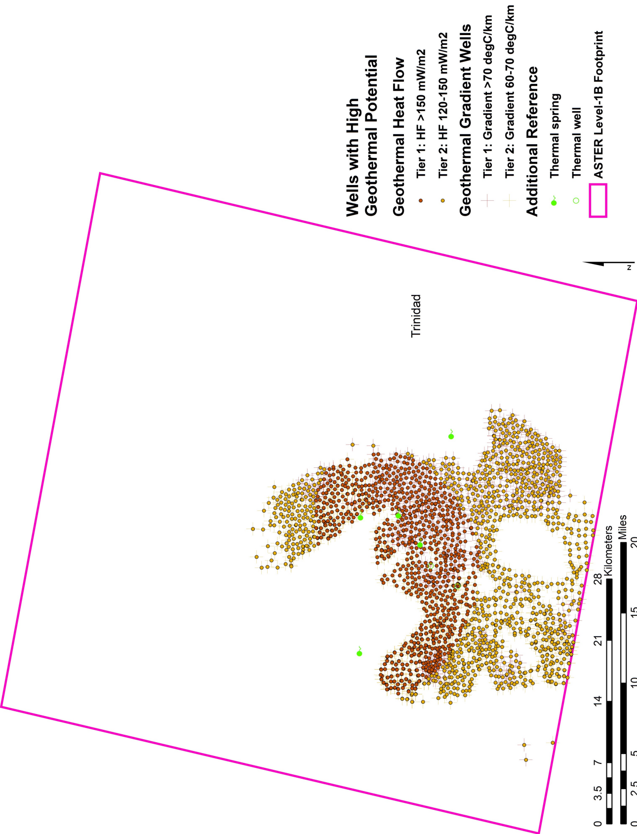
Figure 3. Selected image footprint and Tier 1 and 2 wells near Trinidad, CO. Tier 1 wells are the top ~2% of wells for each of the geothermal properties (gradient and heat flow), Tier 2 wells represent the top ~5% for both gradient and heat flow. An SQL query was run to only include wells that were both Tier 1 and Tier 2 in either thermal gradient or heat flow.
