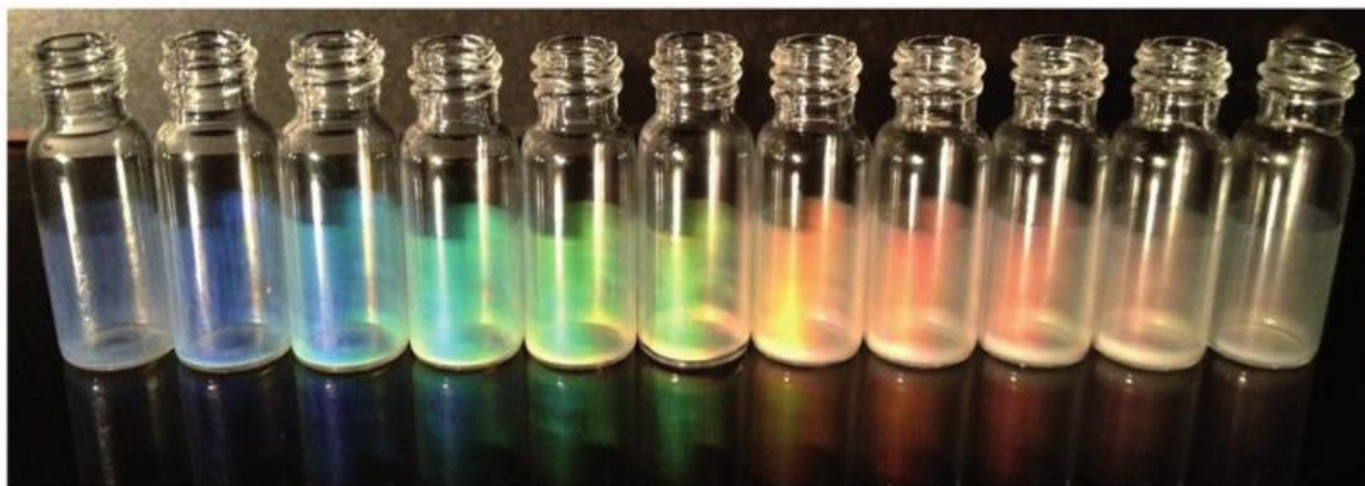
Figure 1. Bottle-brush copolymer blends self-assembled to photonic crystals. Different compositions enable interactions with the full range of visible light. 39
