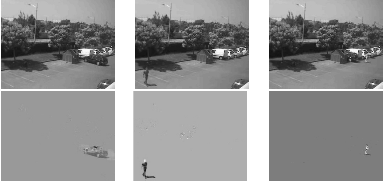
Figure 1.9: Real-time background subtraction using Split-SPCP. Split-SPCP correctly identifies (left) a car in the middle-ground, (center) a person in the foreground, and (right) a person in the background. The resolution is 240 \times 320 pixels per frame, 600 frames were decomposed at one time, and only 200 iterations were allowed.
