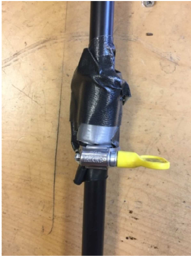
Figure 3 Pole shaft with lead strip resting on a hose clamp that was tightened to the pole shaft at the center of mass of the pole shaft
