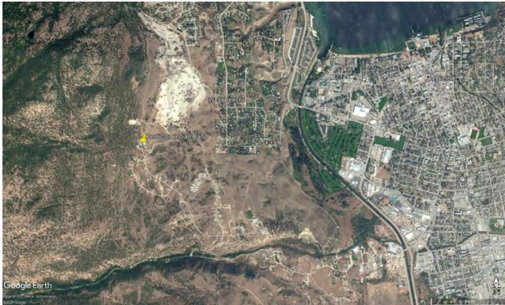
Shadows of utility poles indicate above-ground electricity, like the sample houses in nearby Penticton. Foliage is sparse and set back far enough from roads to suggest that power lines generally have 5 metres of clearance to vegetation, unlike most of the sample houses in Penticton. Images are not clear enough to check the presence of fire hydrants. There are no obvious water bodies from which to draft.
