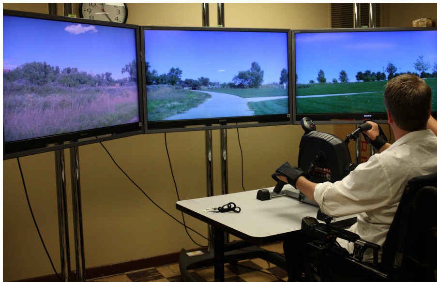
Figure 2.15: Three Screen VEE playback System with an Ergometer at the Focus Group
