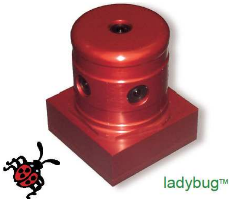
Figure 5.18: Ladybug panoramic camera with 6 small image sensors, courtesy of PointGrey.
