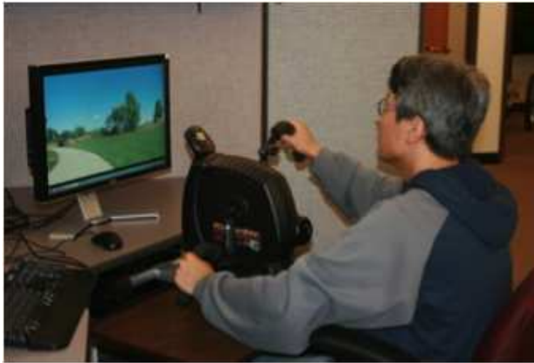
Figure 2.12: One Screen Setup of the Second Generation VEE Playback System with a Desktop Ergometer
