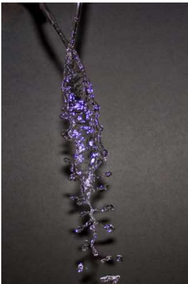
Figure 4.2: Image by students Emily Howard, Preston Wheeler; Colliding water jets result in a 'fishbone' instability, 2012.
