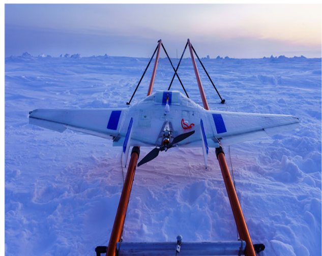
Figure 1.2: DH2 UAS prepared for launch during Multidisciplinary drifting Observatory for the Study of Arctic Climate (MOSAIC) campaign (2019).
