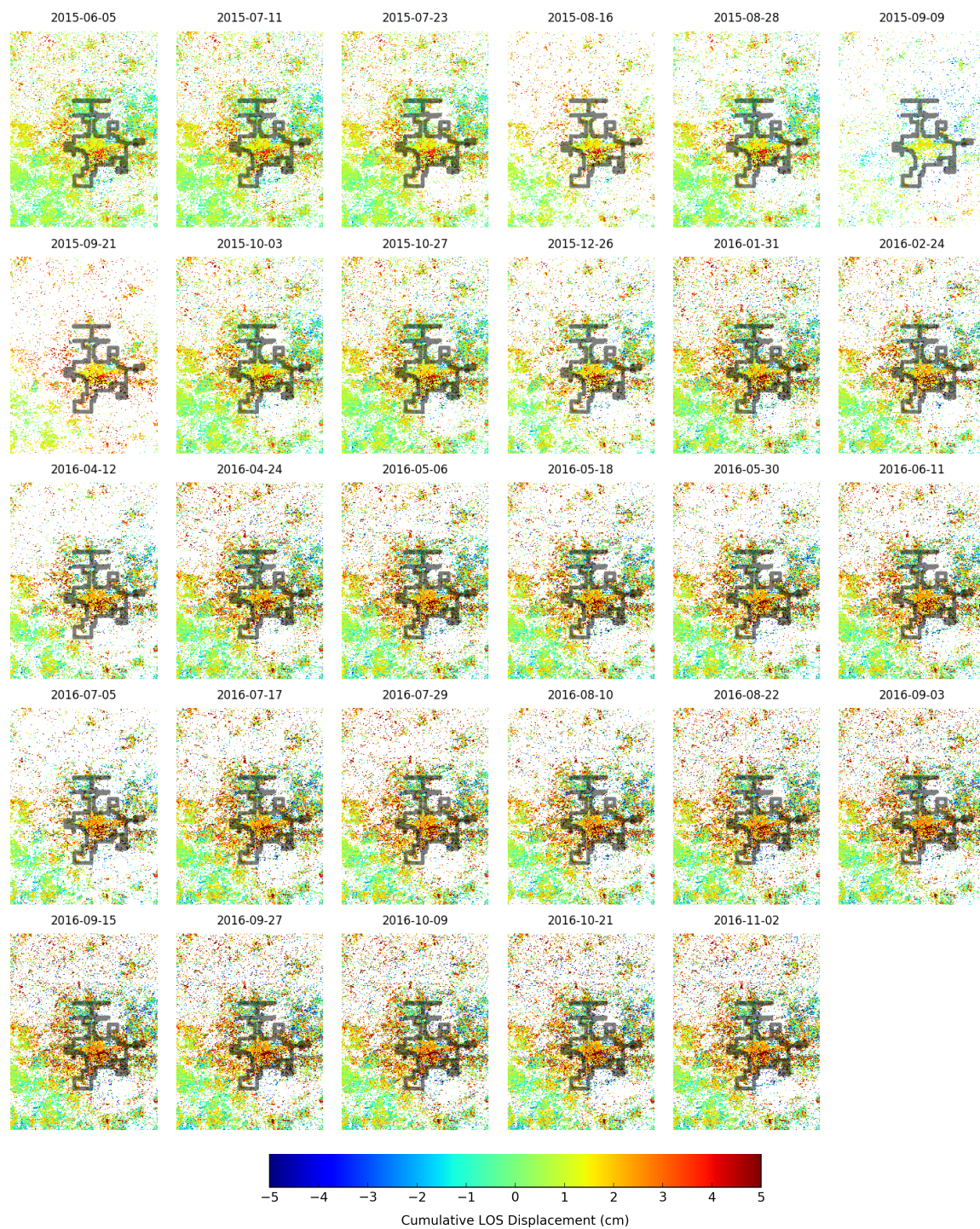
Figure 14. Cumulative displacement time series slices overlaid with Cushing city boundary (gray outline).
