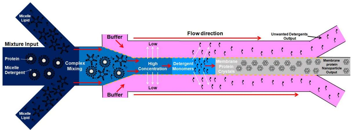
Figure 6.1 Example of membrane protein nanoparticle formation with mixing function. The protein sample with micelle detergent can be adjustably mixed with lipid by using controllable syringe pump.
