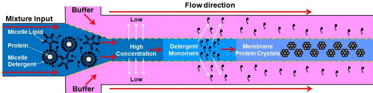
Figure A.1. Diagram of the flow focusing in microfluidic channel.
