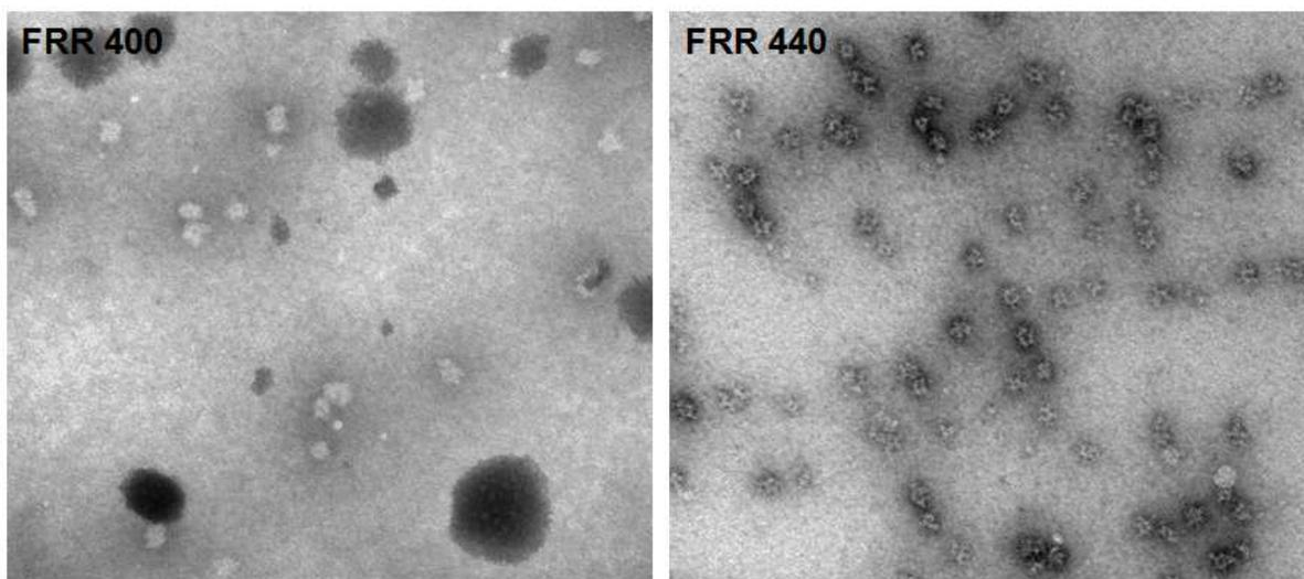
Figure 4.13 shows the repeat result of membrane protein lipid nanoparticle occurred between FRR 400 to 440 with increased 5 times concentration.
