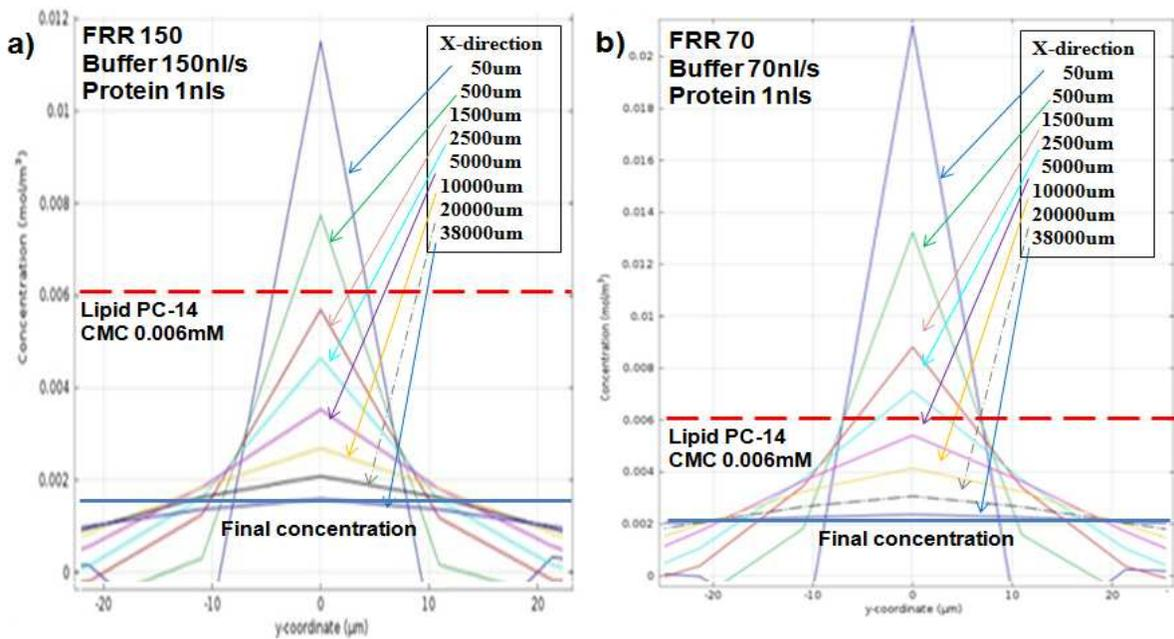
Figure 4.7 the left diagram shows the distribution of lipid PC-14 concentration when FRR at 150. The center flow concentration is mostly lower than its CMC that means lipids become monomer
