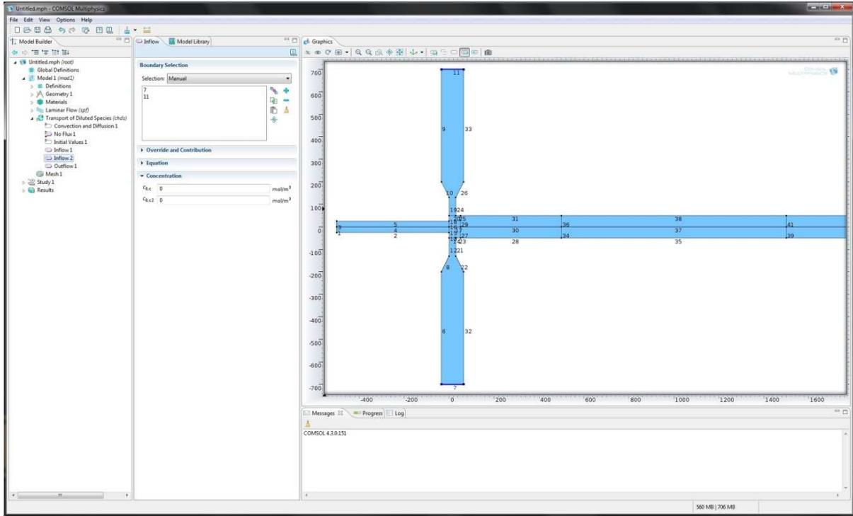
Figure A.14 shows how to define the inflow 2 inlet and initial concentration.
