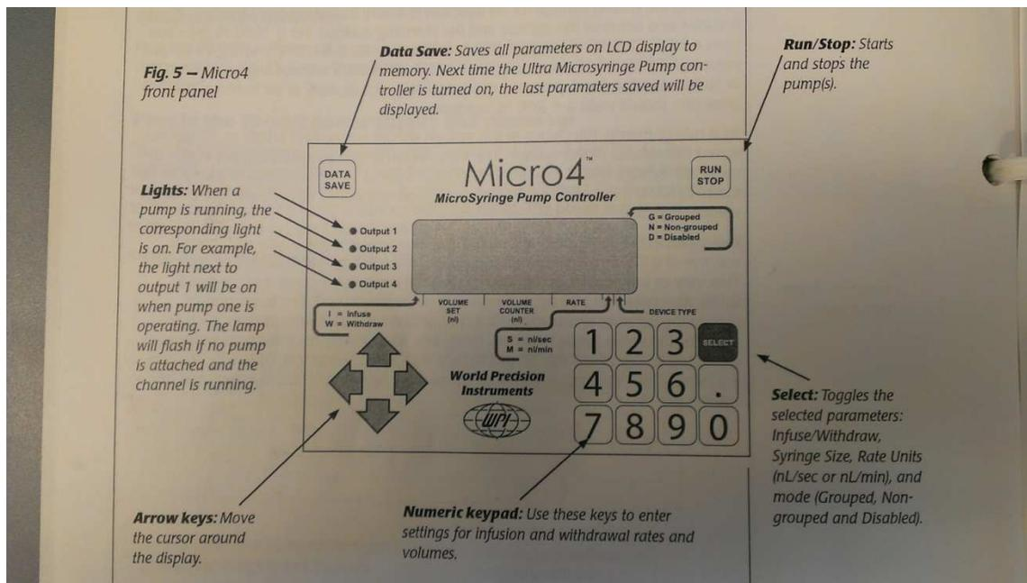
Figure B.5 shows the functions on the control panel of the main controller for controlling each individual syringe pump.
