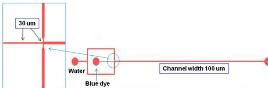
Figure 3.9 The experimental device for the study on membraneless laminar flow. The channel widths are 100 $\mu$ m for the main mixing channel and 30 $\mu$ m for T-junction channels.
