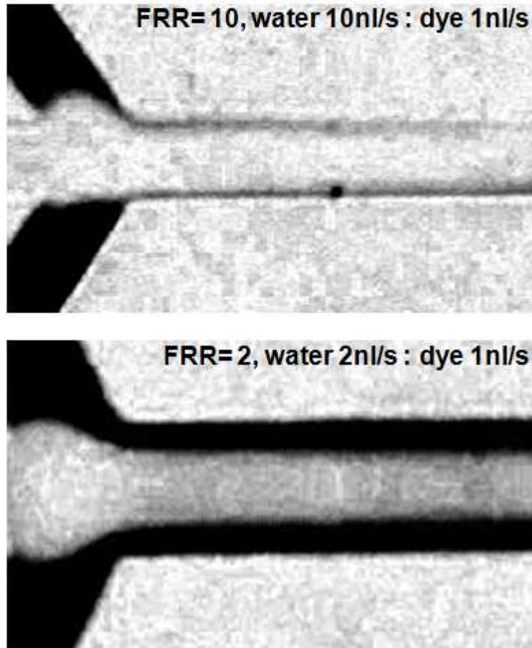
Figure 5.3 shows the close view of mixing zone in blue dye test. Top image is flow pattern in mixing zone when FRR of water and dye is 10. Bottom image is the flow pattern when FRR of water and dye is 2.
