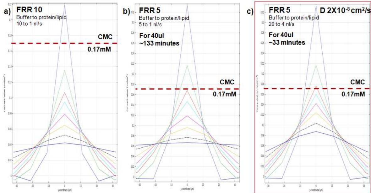
Figure 5.8. shows the concentration distribution of detergent *n*-dodecyl- $\beta$ -D- maltopyranoside (DDM) in microfluidic channel. a) when FRR at 10 with buffer solution 10nl/s and protein/lipid sample 1nl/s, b) when FRR at 5 with buffer solution 5nl/s and protein/lipid sample 1nl/s, c) when FRR at 5 with buffer solution 20nl/s and protein/lipid sample 4nl/s.
