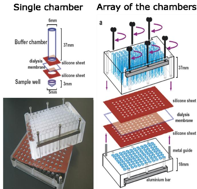
Figure 2.5 shows currently the common method for 2D membrane protein crystallization. The equipment consists of buffer chamber on the top, dialysis membrane in the middle, and sample well at the bottom. Detergents will be removed to buffer chamber by natural diffusion process and dialysis membrane will keep the large molecules in sample well [26].
