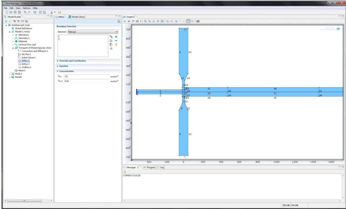
Figure A.13 shows how to define the inflow 1 inlet and initial concentration.
