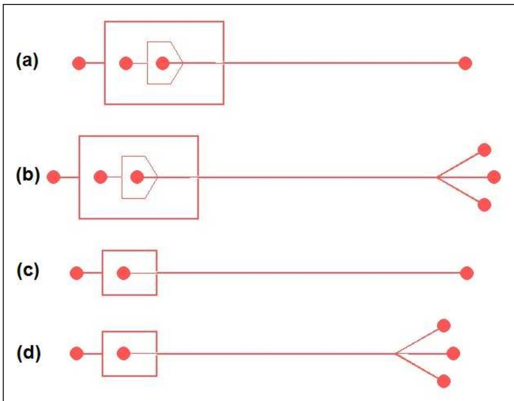
Figure 3.1 shows the global view of four designs, top to bottom are a mixing device, mixing device with designed outlet for increasing density, flow focusing lamina flow device (c), and flow focusing lamina flow device with designed outlet for increasing density (d).
