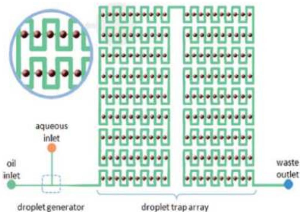
Figure 1.6 shows the scheme of the microarray by using the flow resistance concept. Eventually droplets located and isolated in each trap for experiment [16].
