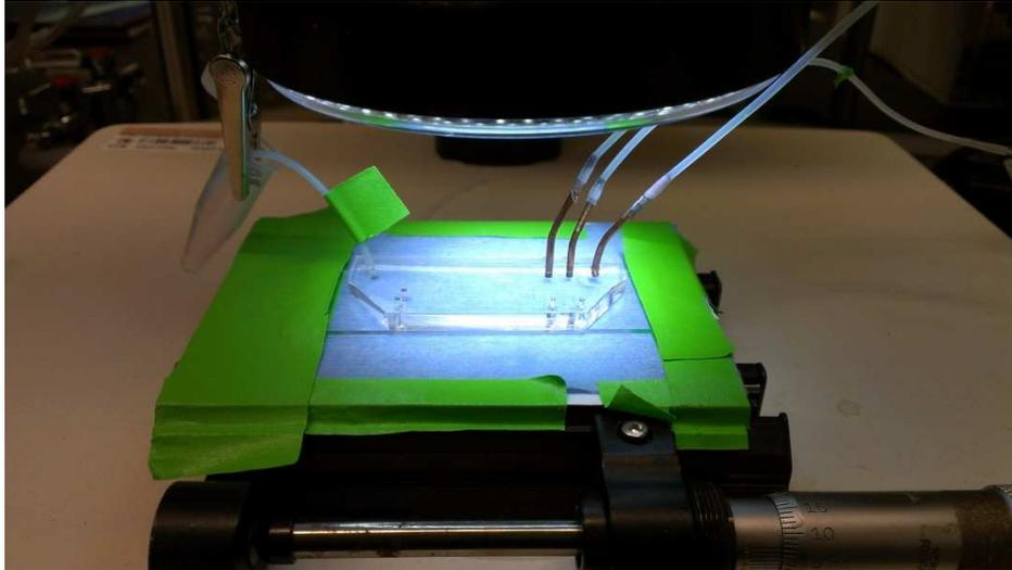
Figure B.3 shows the tubes connected from syringe pump to inlets(right) and outlet(left) of PDMS microfluidic device.
