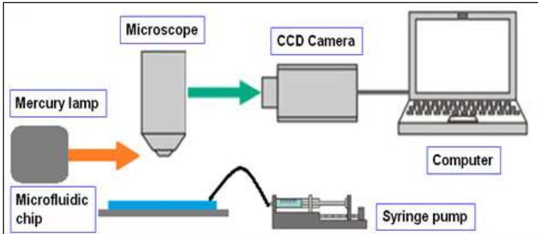
Figure 3.7 shows the experiment set up which consists of syringe pumps with a controller that can precisely adjust the flow rate down to  $1\text{nl/m}$  and a CCD camera with a microscope to capture images for data analysis.
