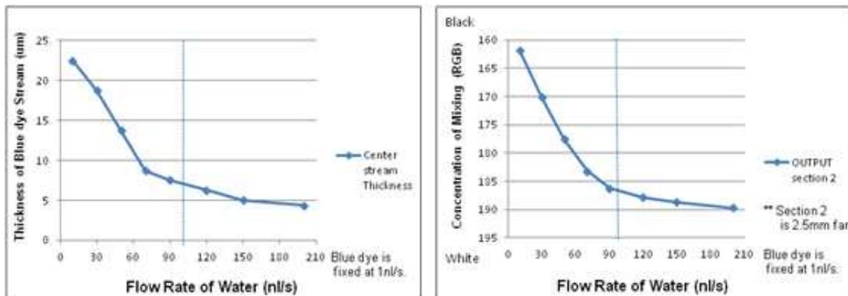
Figure 3.12 shows the different thickness of blue dye stream changed with various FRRs in left diagram. A higher FRR has thinner thickness of blue dye inducing fast diffusion due to the large surface to volume ratio. The right diagram shows the increasing flow rate ratios gradually diminished concentration with faster diffusion speed.
