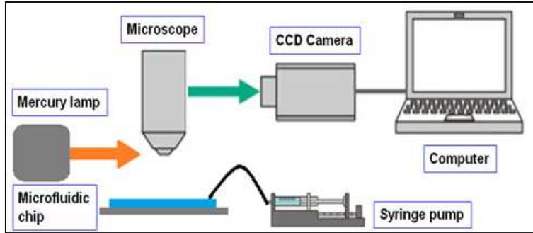
Figure B.1 shows the equipments of the entire experiment set up.
