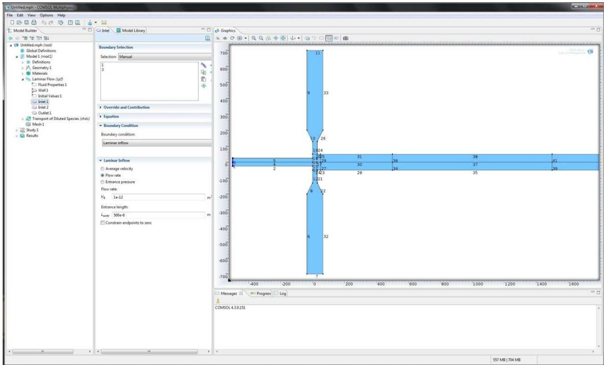
Figure A.10 shows how to define the inlet for liquid input.
