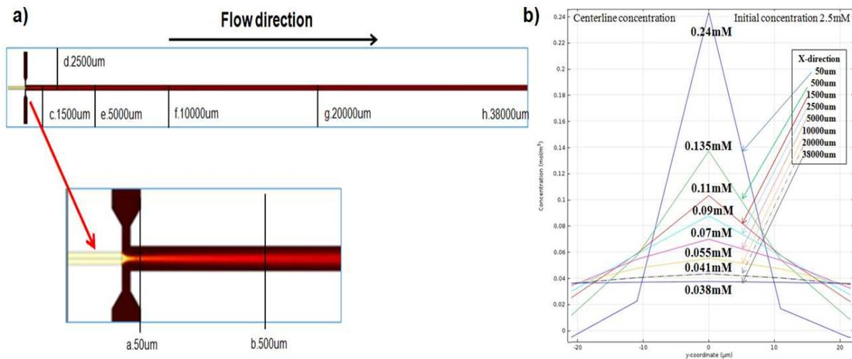
Figure 4.5. a) shows the total 8 measuring points at different distance in X-direction from 50μm to 38000μm. b) shows the distribution of center flow concentration at different measuring points.
