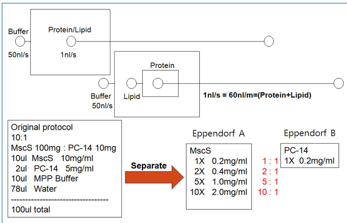
Figure 5.5. shows the illustration of mixing ratio for protein/detergent sample and lipid applied to individual input of mixing chip. The protein to lipid ratio in previous study were 10 to 1 (2mg/ml : 0.2 mg/ml). In this mixing chip experiment, they being separated into two individuals eppendorf A for MscS and eppendorf B for lipid PC-14.
