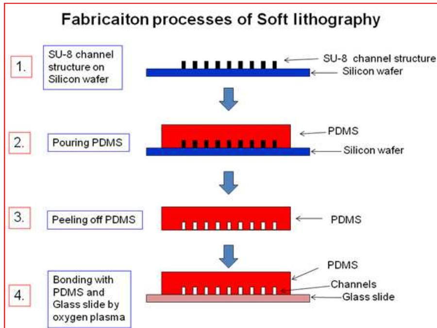
Figure 3.4 Fabrication Processes of Soft lithography. 1. Preparation of SU-8 channel structure on silicon wafer. 2. Carefully pour PDMS on silicon wafer avoiding bubbles. 3. Peel off PDMS from silicon wafer. 4. Bonding PDMS with glass slide by using oxygen plasma.
