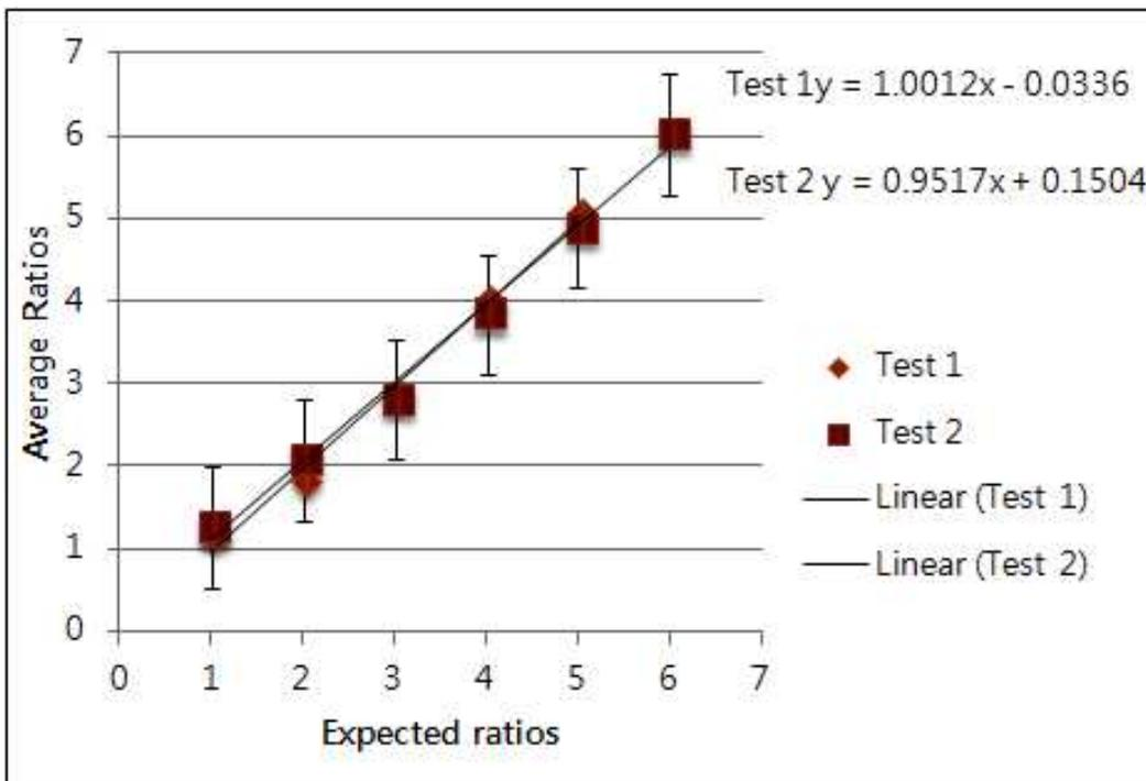
Figure 5.4 shows the result of mixing ratio stable test that two experiment results are both nearly linear lines from mixing rate are 1:1 to 6:1.
