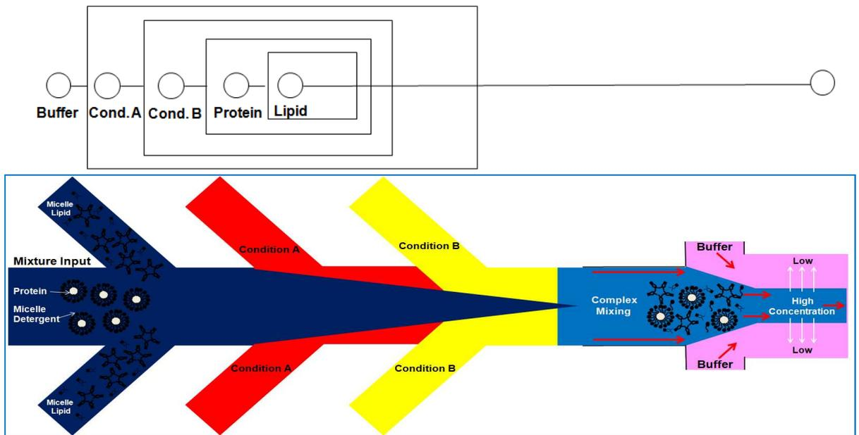
Figure 6.2 shows the multi-input microfluidic device design for verifying the possible combinations of different conditions such as protein to lipid ratio, ph, and salt concentrations.
