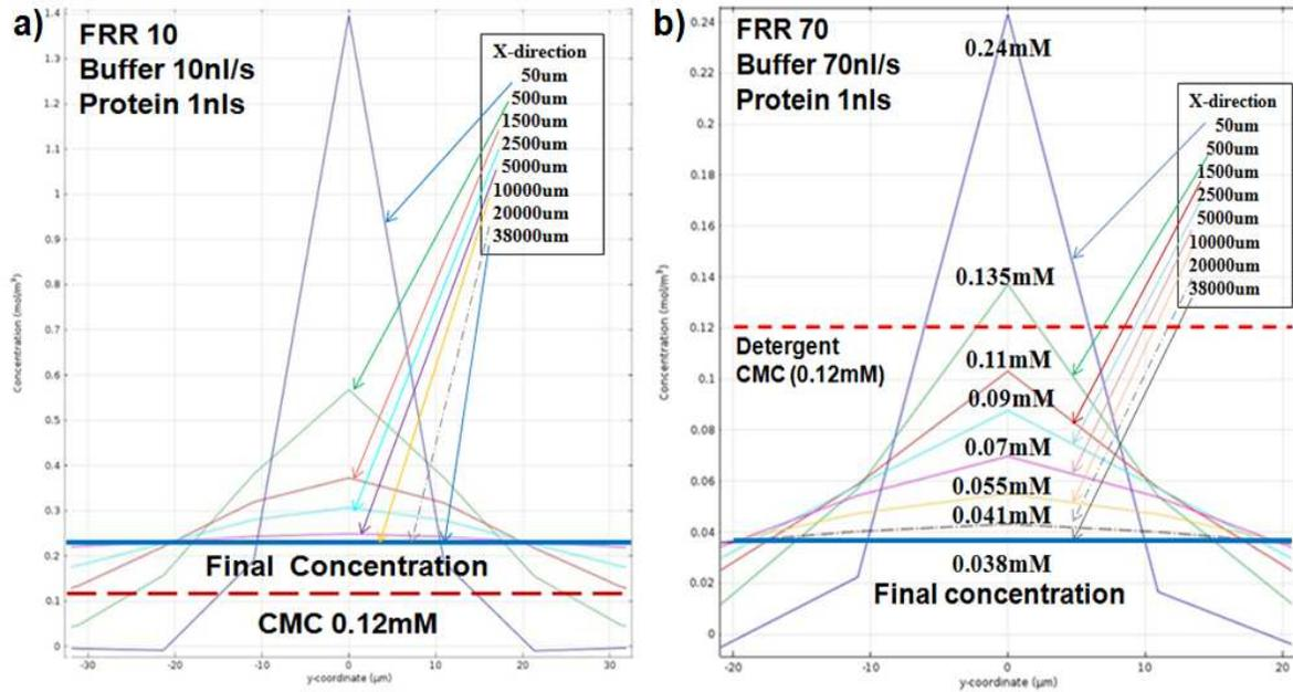
Figure 4.6 the left diagram shows the distribution of detergent FC-14 concentration when FRR at 10. The final concentration is higher than its CMC that means detergents are still in micelle formation. The right diagram shows the distribution of detergent concentration when FRR at 70. The final concentration is smaller than CMC which means the detergents form monomer structure.
