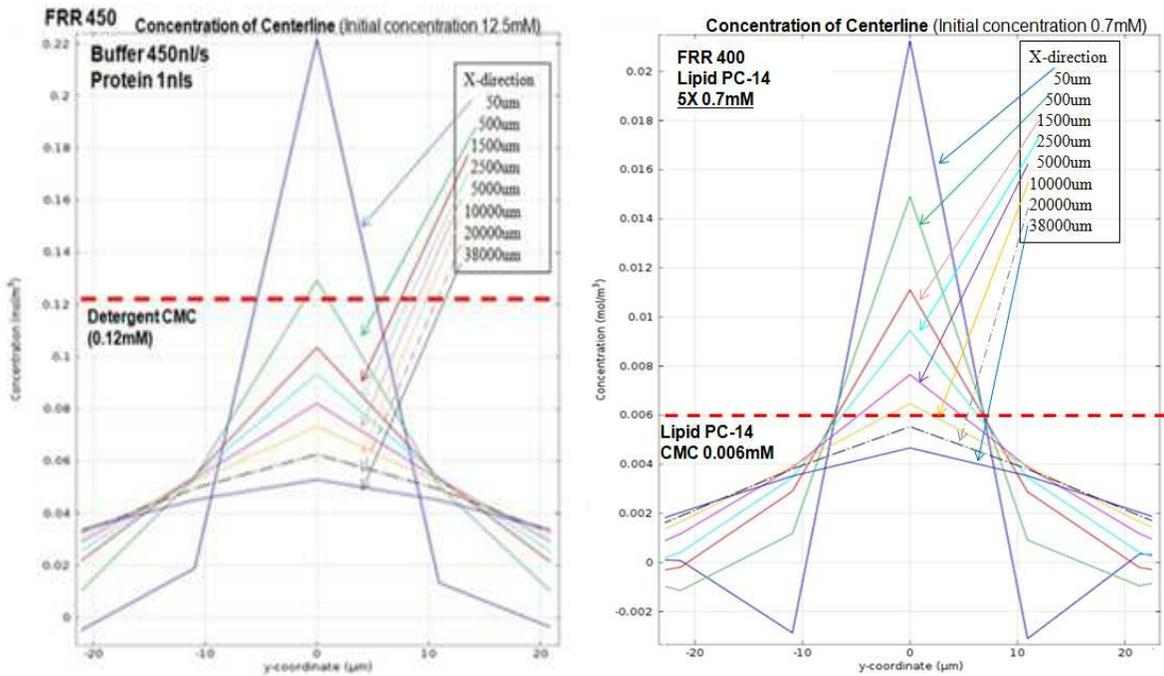
Figure 4.11 shows in the left diagram the simulation result of the distribution of detergent concentration at the FRR of 450 at 5 times more concentrations of detergent; right diagram shows the simulation result of the distribution of detergent concentration at the FRR of 400 at 5 times more concentrations of lipid increased. In this case, the initial concentrations of detergent and lipid are 12.5mM and 0.7mM.
