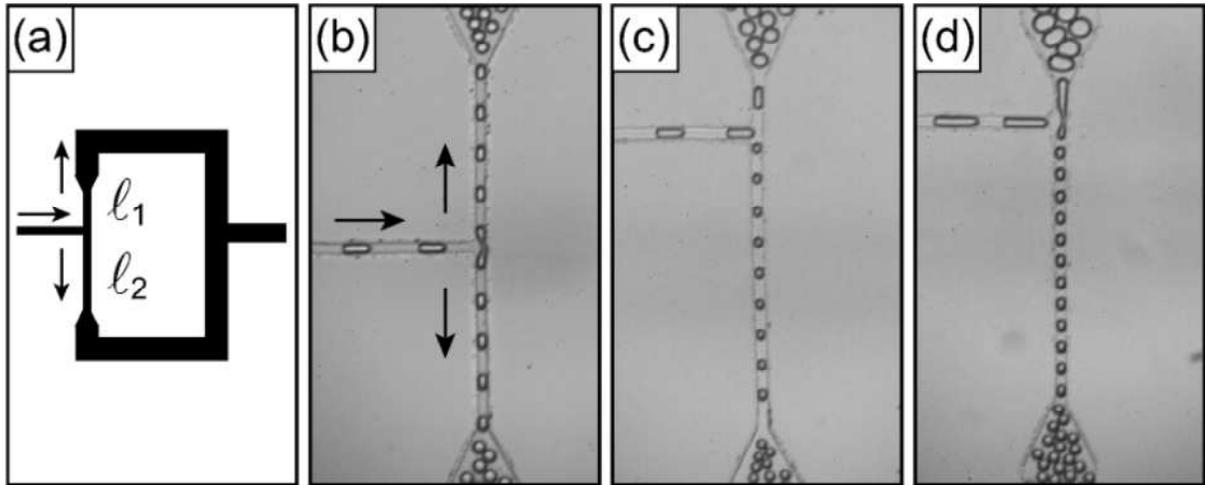
Figure 1.4 shows the method of the droplet break up in T-junction. b) same lengths of channels with same break up droplet size; c,d) longer length of channel has smaller droplet due to higher flow resistance [13].
