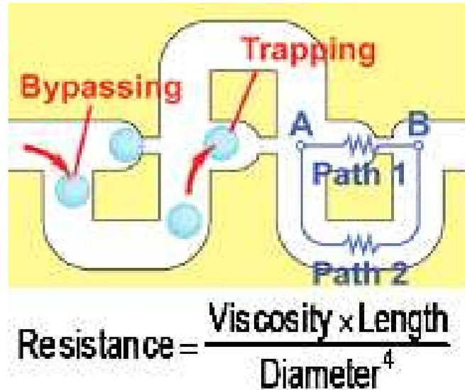
Figure 1.5 shows the schematic and equation of the flow resistance. The droplet is delivered and localized into a trap with two paths, path 1 and path 2. The droplet will choose path 1 and after it is localized. The following droplet will bypass through path 2 and sit in the next trap [14].
