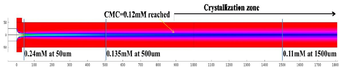
Figure 4.8 shows numerical simulation of a successful crystallization run (FRR=70) with the micelle detergents encapsulating proteins disassembled into monomers at around 900  $\mu\text{m}$  along the mixing channel with a total length of 38,000  $\mu\text{m}$ .
