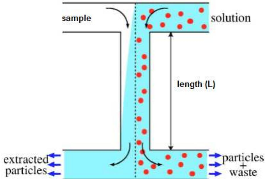
Figure 1.7 Presents a membraneless H filter. Sample and solution with particles mixed in initial intersection of main channel. The lack of diffusion length ( $L$ ) does not allow time for particle to diffuse. Thus the particles remain in the initial stream and are delivered to the waste outlet. The sample with purified solution without particles is sent to the outlet of left-hand side.
