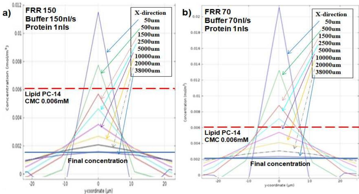
Fig 5.9. the left diagram shows the distribution of lipid PC-14 concentration when FRR at 150. The center flow concentration is mostly lower than its CMC that means lipids become monomer structure. The right diagram shows the distribution of lipid concentration when FRR at 70. The concentration is larger than its CMC meaning that the lipids retain a micelle structure.
