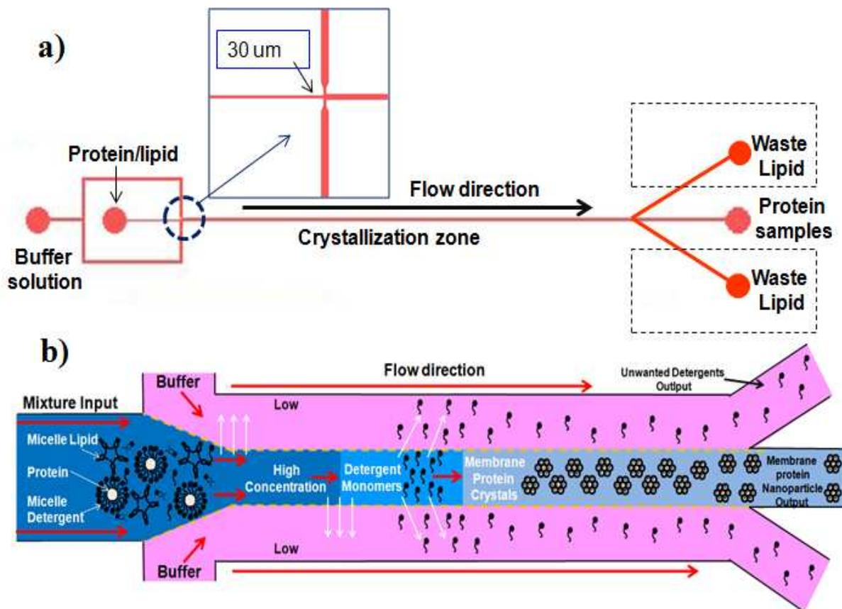
Figure 4.16. a) shows a channel design with one output for the collection of protein samples and two additional outputs for the removal of unwanted detergents. b) shows the microfluidic device developed for membrane protein nanoparticle formation accomplished by adding two additional outputs.
