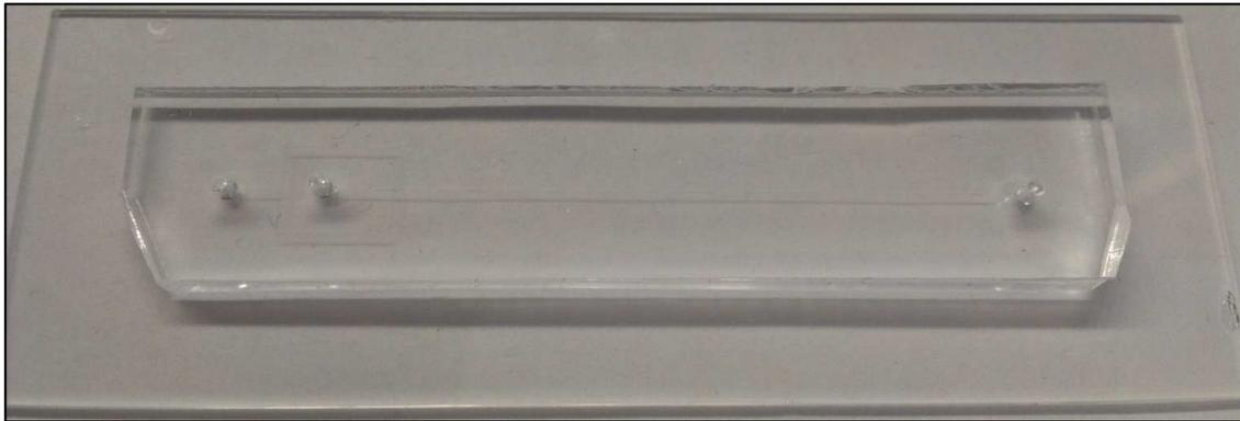
Figure 3.6 shows the image of the microfluidic device that PDMS bonds with glass slide
