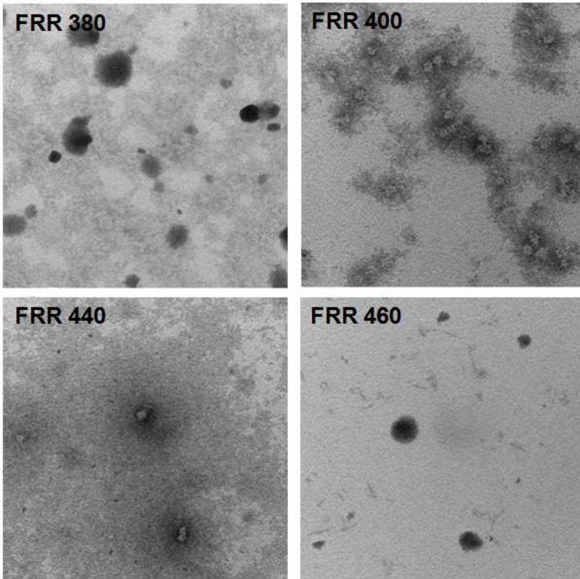
Figure 4.12 shows the FRR test results from 360 to 460. No nanoparticles found when FRR is smaller than 380 and larger than 440.
