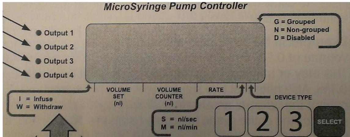
Figure B.6 show the closer view of display panel where has infuse/withdraw, volume set, volume counter, rate (nl/sec, nl/min), and device type.
