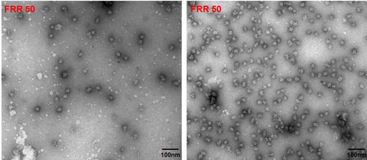
Fig. 4.17. presents the density of membrane protein nanoparticle increased by modifying the output design. The left image shows the result of the nanoparticle density from a single output. The right image shows the result with two extra outlets that can remove unwanted detergents and buffer solution. Approximately, the density of membrane protein nanoparticle in new output design has been increased 40%.
