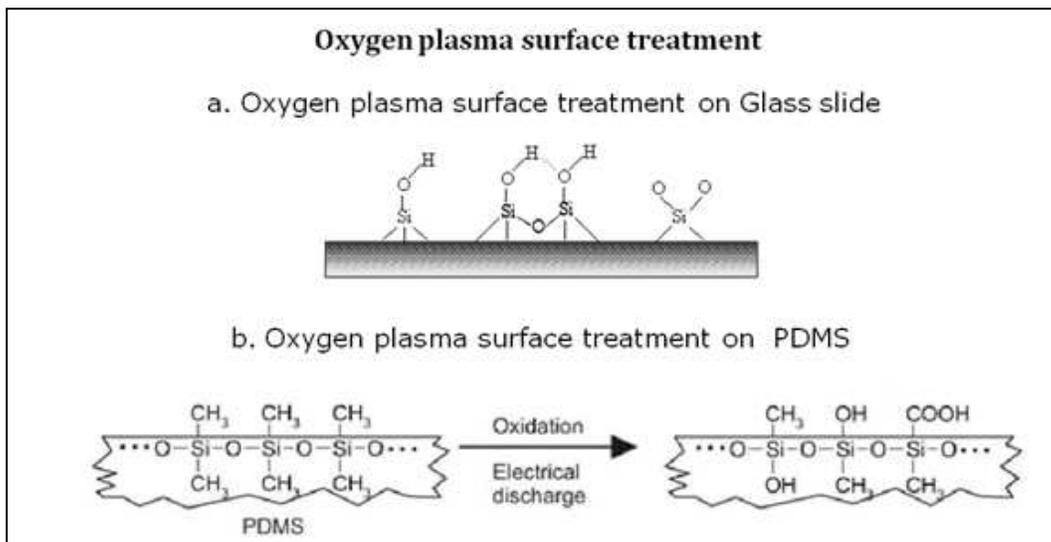
Figure 3.5 shows the chemical reactions of glass slide and PDMS after oxygen plasma surface treatment. Glass slide after surface treatment will obtain OH on the surface and reactive a Si-O covalent bonding interface with treated PDMS.
