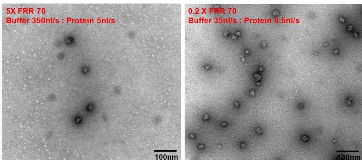
Figure 4.15 illustrates the EM image results of the membrane protein nanoparticles generated by same FRR of 70 with different flow speed. The left image shows few nanoparticles generated by “5X faster” (buffer 350nl/s ; protein 5nl/s) than the original FRR of 70 (buffer 70nl/s ; protein 1nl/s) ; The right image shows more uniform nanoparticles generated by “5X slower” (buffer 35nl/s ; protein 0.5nl/s) than the original FRR of 70.
