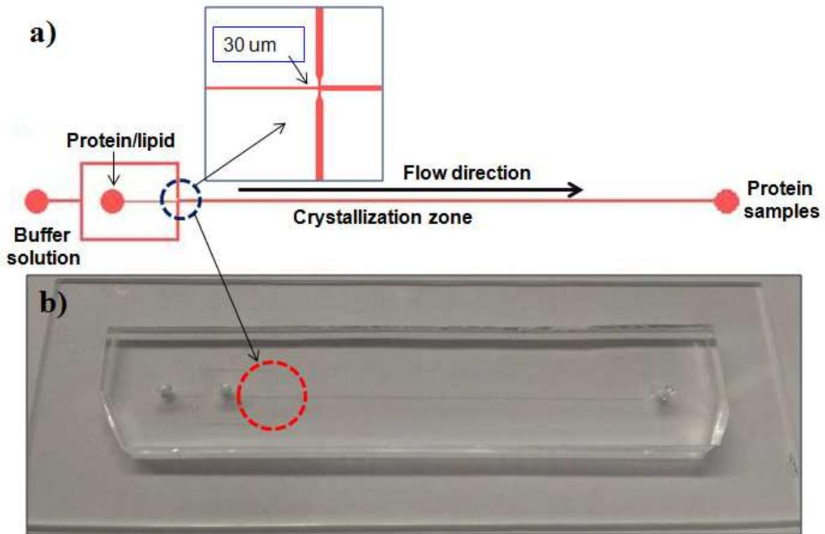
Figure 4.2 a) Channel design pattern that is accomplished by using controlled flow focusing to boost the crystallization process and additional outputs for removing unwanted detergents, b) Device image shows the exact chip size as same as glass slide.
