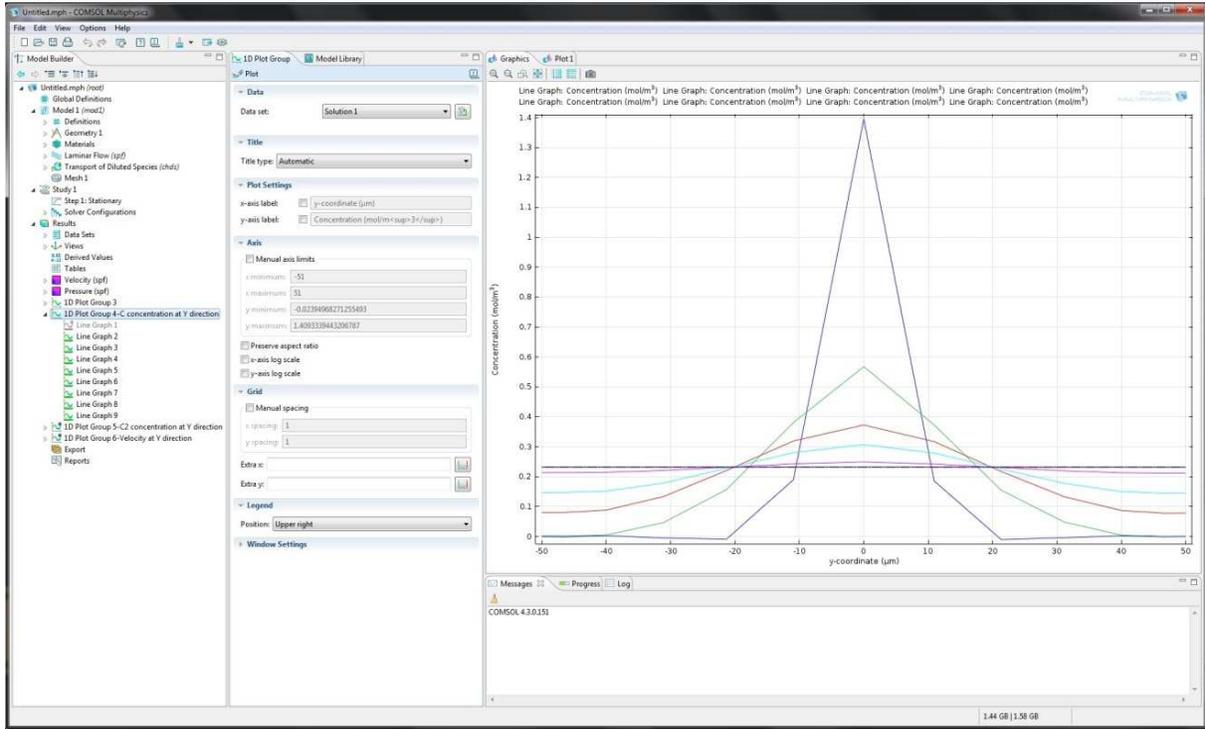
Figure A.20 shows the 1D plot for Detergent concentration distribution of cross-section along the vertical direction
