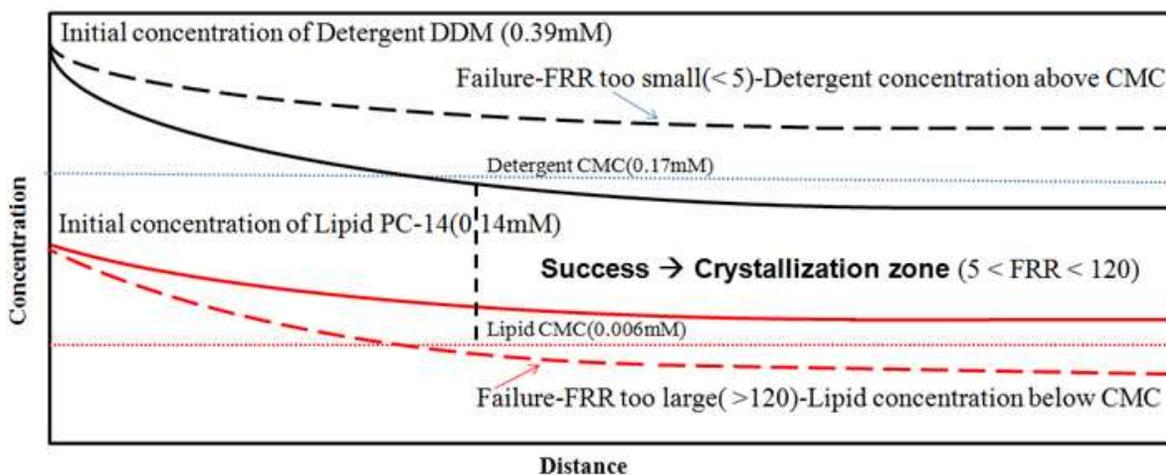
Figure 5.10 shows the estimated crystallization zone from the simulation result that indicates the possible FRR range for successfully forming the membrane protein nanoparticles. The minimum FRR is 5 and the maximum FRR is 120.
