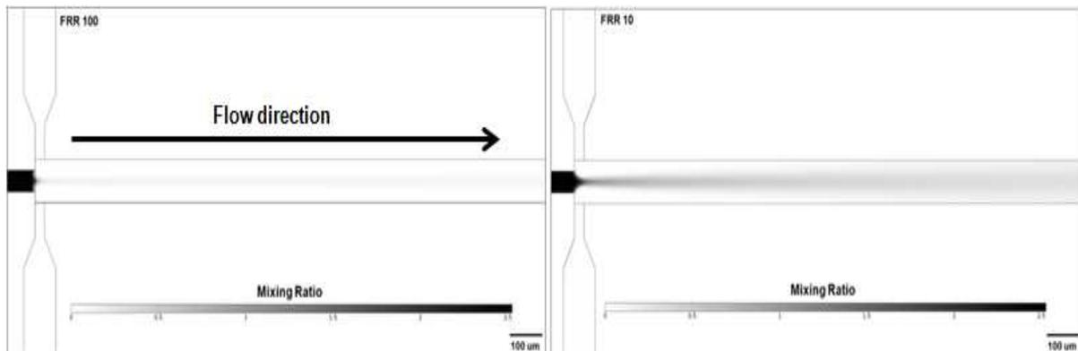
Figure 4.4 shows the numerical simulation results for flow focusing laminar flow in microfluidic channel. The left image shows the concentration diffusion distribution of a flow rate ratio of 100 with a thin center stream. The right image shows another case of flow rate ratio of 10 with a thick center stream.
