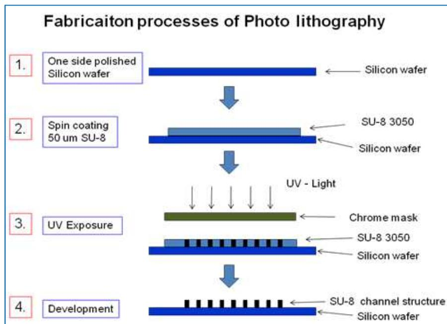
Figure 3.2 Fabrication processes of photolithography. 1. Preparation of one-side polished silicon wafer. 2. Pour SU-8 on the top of silicon wafer and spin coating at certain speed. 3. UV exposure. 4. Development for removing un-crosslinked SU-8.
