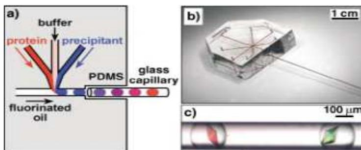
Figure 1.2 shows the mixing with buffer, protein and precipitant with different conditions and formed droplets by continuous oil in T-junction. Then droplets are delivered to glass capillary for X-ray screening [9].
