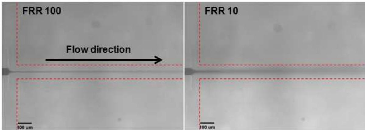
Figure 3.11 The laminar flow in the microfluidic channel. The thickness of the dye flow is controlled by changing the water-to-dye flow rate ratio (FRR). The left image shows a case with a flow rate ratio of 100, the dye stream was very thin. The right image shows another case with a flow rate ratio of 10 with a thick dye stream. The red dashed line represents the physical walls of the device.
