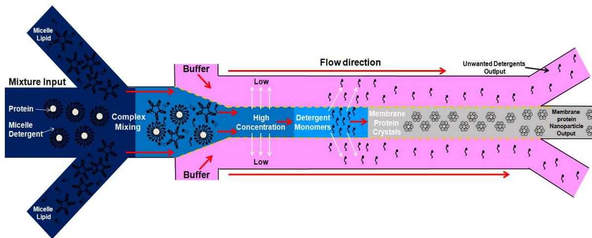
Figure 5.1 Example of membrane protein nanoparticle formation with mixing function. The protein sample with micelle detergent can be adjustably mixed with lipid by using controllable syringe pump.
