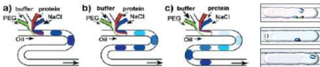
Figure 1.1 shows a microfluidic system for protein crystallization. (a-c) gradient droplet colors present each protein sample has different conditions by controlling flow rate. (e) Protein crystallizes [8].
