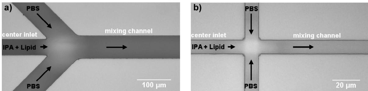
Figure 1.9 presents the flow focusing method applied on forming a lipid vesicle. The higher concentration of lipids were diluted by convection-diffusion and belloved its CMC to reconstitute vesicle structure.
