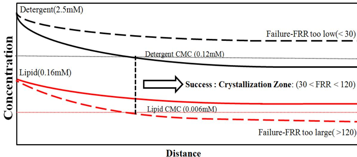
Figure 4.10 shows when the FRR is too low, the crystallization would fail because the concentration of the micelle detergents could not reach levels lower than the CMC of 0.12mM required for releasing the proteins. When the FRR is too high, the crystallization would fail also because the concentration of the micelle lipids could quickly reach levels below the CMC of 0.006 mM and become lipid monomers.
