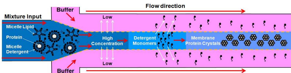
Figure 4.1 Examples of successes in membrane protein crystallization by a conceptual breakthrough using controlled convective-diffusive transport in microfluidic channel to boost the crystallization process. The interfaces between the center mixture and the side buffer streams can create concentration gradients where detergent can be removed and membrane protein aggregated with lipids to form the nanoparticles
