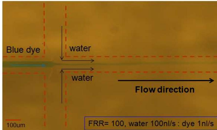
Figure 3.10 shows the flow pattern of flow focusing at FRR of 100. The water flows being injected from both perpendicular sides into the main channel and the dye flow being injected into the middle of the main channel
