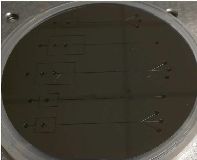
Figure 3.3 shows the illustration of the SU-8 structure on the silicon wafer.
