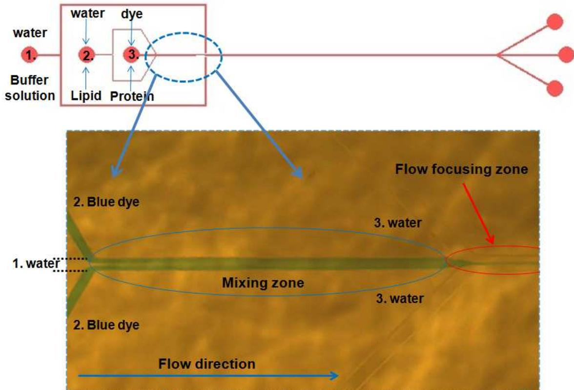
Figure 5.2. shows the designed scheme for the mixing chip. There are three inputs for 1. buffer solution/water, 2. lipid/water, 3. protein sample/blue dye. At the beginning, the input 2 and 3 started mixing completely in the mixing zone and then injected to the main channel merging with input 3 to perform a flow focusing phenomena for conductive-diffusive process.
