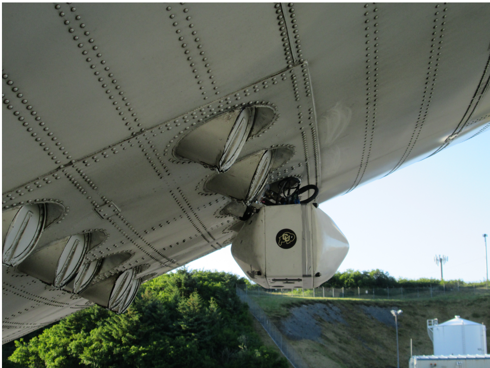
Figure F.2: CULPIS-X Package installed in a flare tube prior to a June 2016 Arctic Flight
