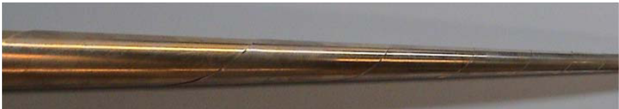
Figure 2.2: Photo of Beryllium copper stacer antenna used in the STEREO mission. The aspect ratio is exaggerated for display purposes and not to scale, meaning that it should be a narrower diameter in practice. Image Credit: Bale et al. (2008).
