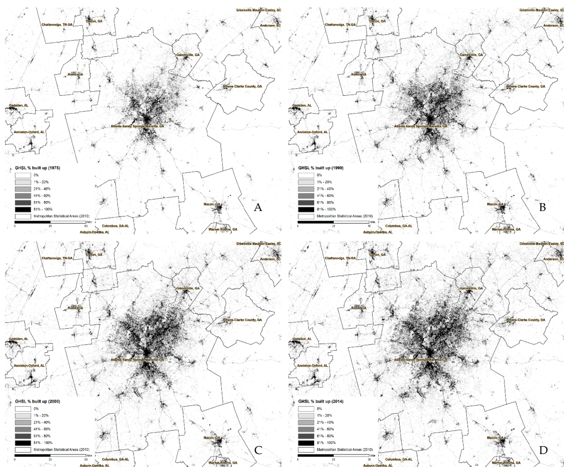
Figure 5. Intensity of built-up land area, as indicated by the Global Human Settlement Layer (GHSL) for the metro Atlanta area in (A) 1975, (B) 1990, (C) 2000, and (D) 2014.
