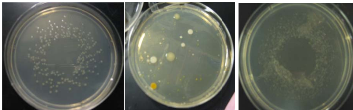
Figure 4-12 Effluent plates. Left picture: inlet, known E. Coli colonies. Middle picture: Effluent plate, unknown bacteria, Right: TNTC
