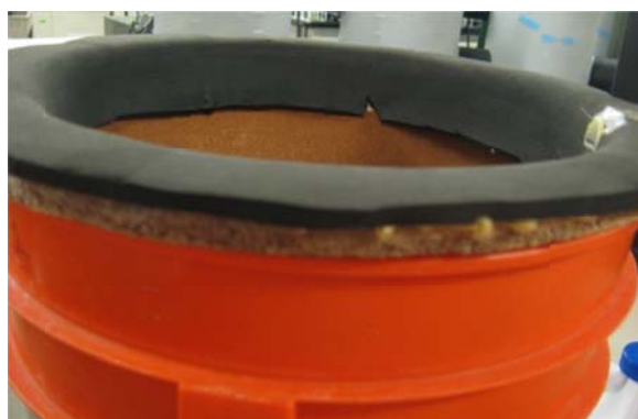
Figure 4-5 Gasket glued to the CPF
