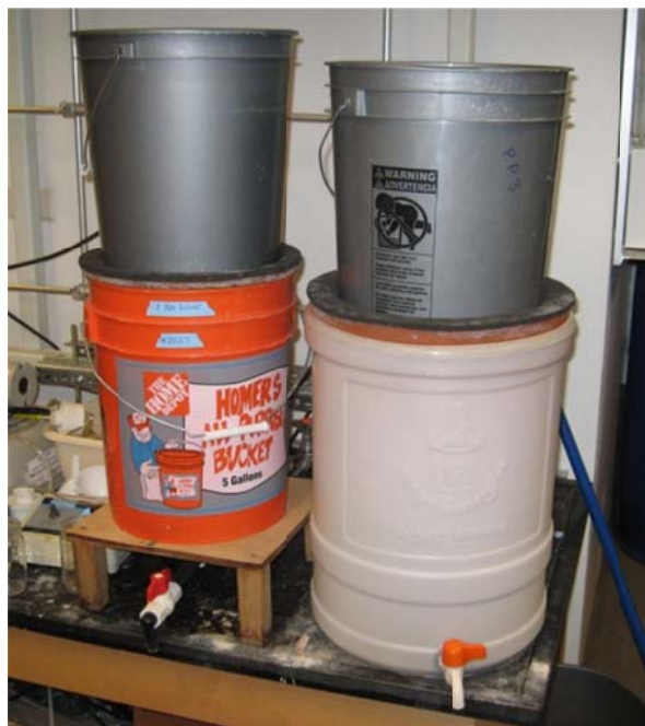
Figure 3-2 Enhanced Ceramic Water Filtration System. Left: Nicaragua ECWF. Right: Cambodia ECWF.
