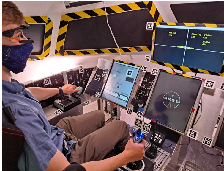
Figure 2.1: Example of participant inside the AReS mockup during a trial. The primary flight display (top), secondary display (left) and reward display (center) are visible. [26]
