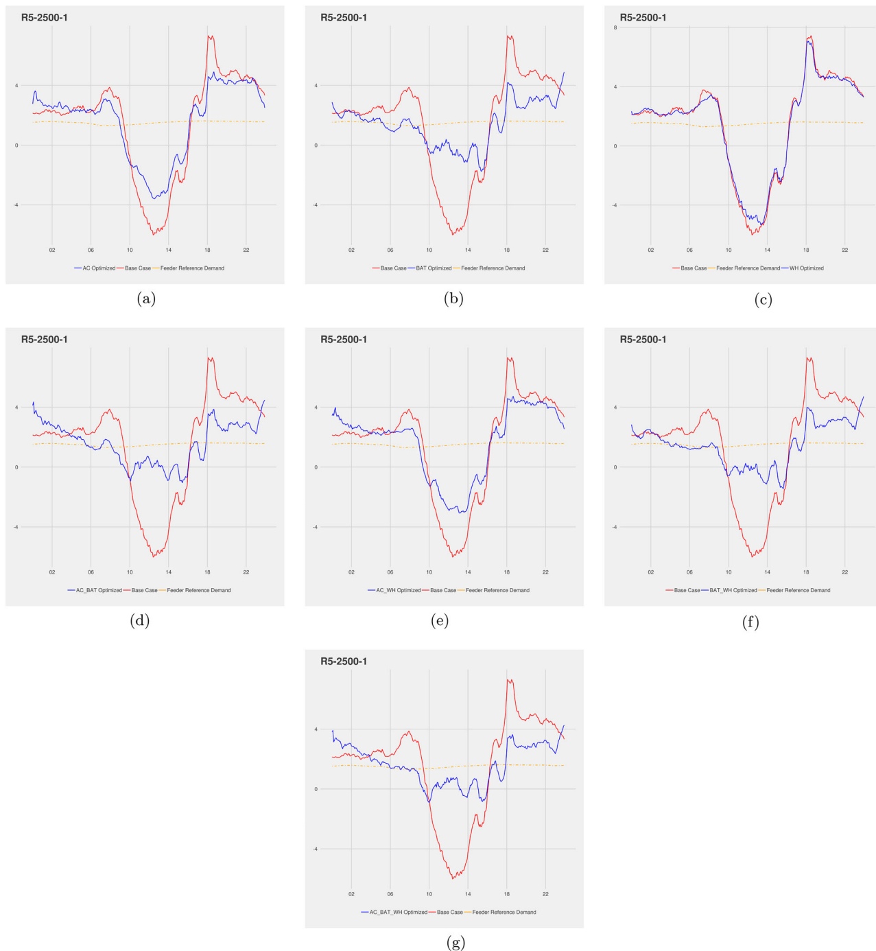
Figure 25. Scenario B load shapes for Houston Feeder R5-2500-1, 23 Aug 2005. load shaping benefits occurred (a) in hours 6–22, and 6, (b) in hours 3–22, and (c) in hours 7 and 13. Complementary load shaping occurred across managed loads in (d) in hours 4–22, (e) in hour 7, (f) hours 3–8 and 19–21, and (g) which had the smoothest optimized load. (a) Air Conditioning. (b) Battery. (c) Water heater. (d) Air Conditioning + Battery. (e) Air Conditioning + Water heater. (f) Battery + Water heater and (g) Air Conditioning + Battery + Water heater.
