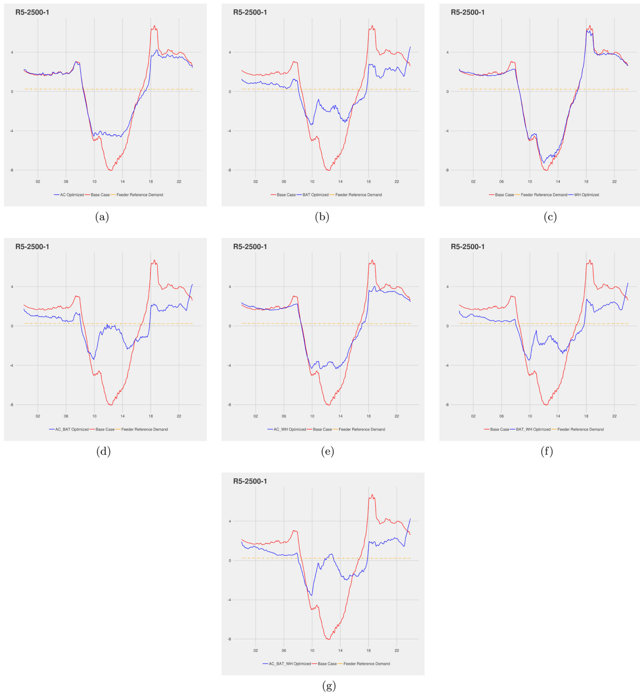
Figure 22. Scenario B load shapes for Houston Feeder R5-2500-1, 18 May 2005. The Feeder Reference Demand was nearly flat. Fifty percent of homes having net-zero PV resulted in mid-day negative generation denoted by the red dip. As expected, GridMPC added load to offset PV generation. Differing performance of load shaping were apparent in (a)–(g). (a) Air Conditioning. (b) Battery. (c) Water heater. (d) Air Conditioning + Battery. (e) Air Conditioning + Water heater. (f) Battery + Water heater and (g) Air Conditioning + Battery + Water heater.
