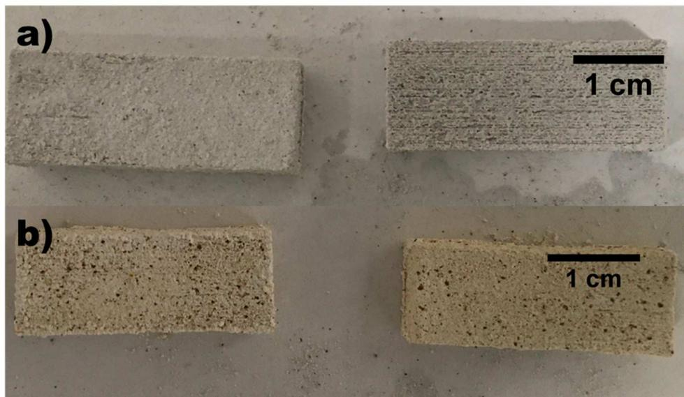
**Figure 22:** Examples of powder binder jet printed bars of simulated lunar regolith MOC cements a) as printed b) after sintering.
