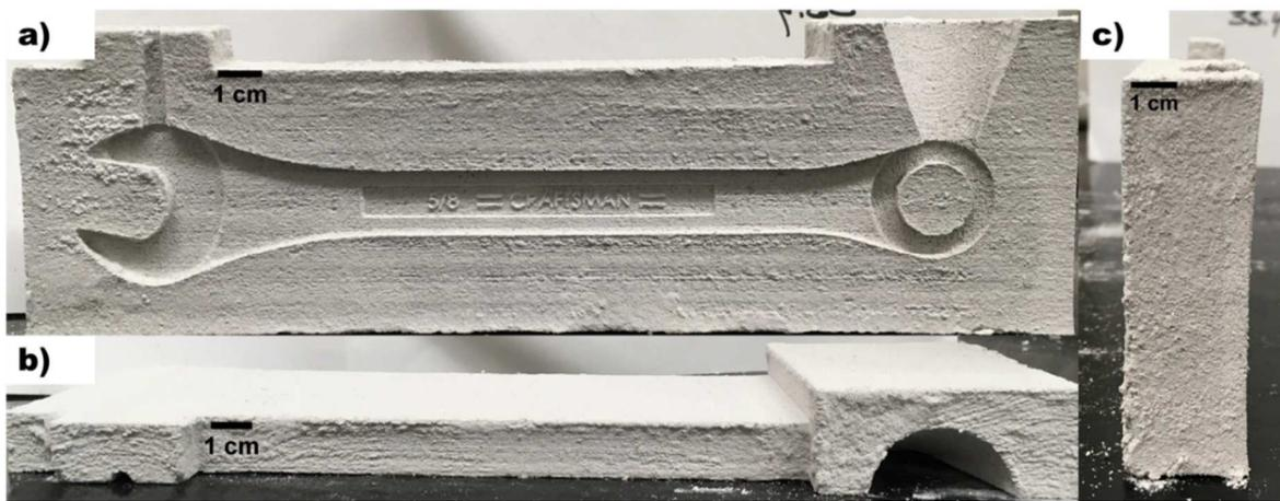
**Figure 23:** Powder binder jet printed wrench mold of simulated lunar regolith MOC cements. a) cross section b) length, and c) width
