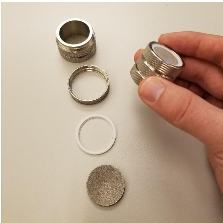
Figure A.11: Oligopilot reactor columns. The 6.3 mL column is fully assembled while the 12 mL column has one end screwed off and the porous frit disassembled to exhibit the inside of the reactor.
