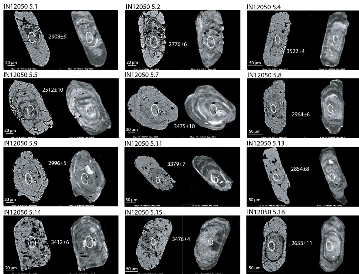
Figure 7. Backscatter electron and cathodoluminescence paired images of zircon grains used in geochronological and trace-element analysis (above: IN12050).
