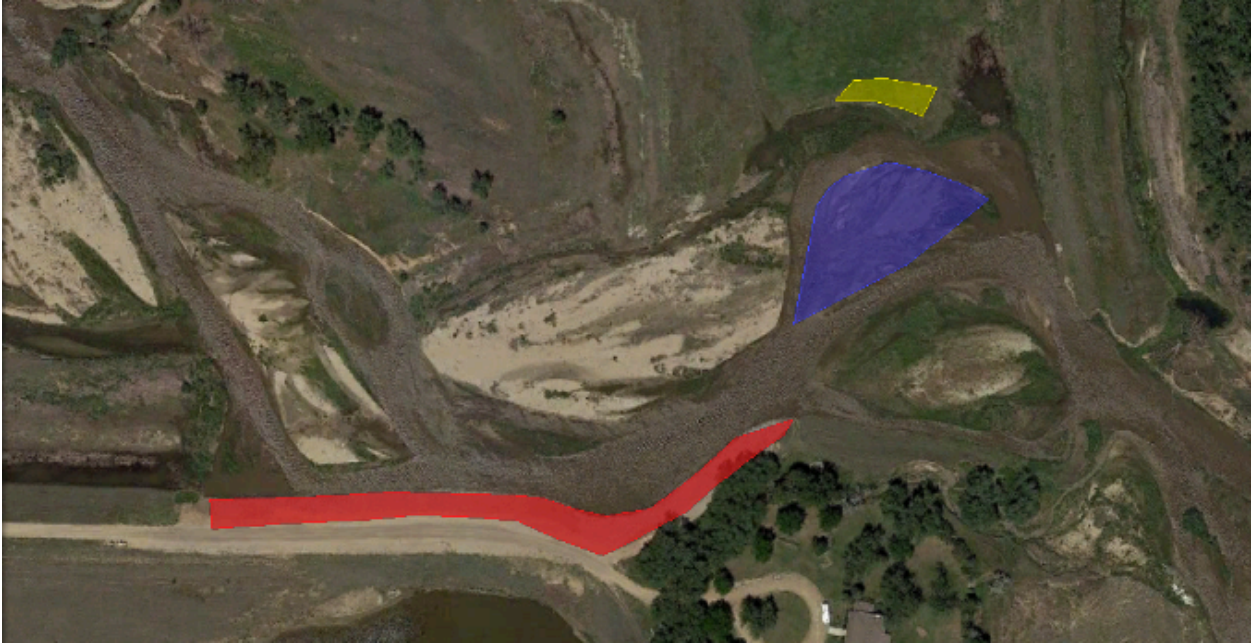
Figure 17 – Image of Study Site 1 in June 2017. Rip Rap structure is highlighted in red. The Sand Bar planting area is highlighted in purple, and the Weedy Bench planting area is highlighted in yellow. Notice the angle at which the stream flow is directed as it flows along the riprap, potentially flooding the restoration area.
