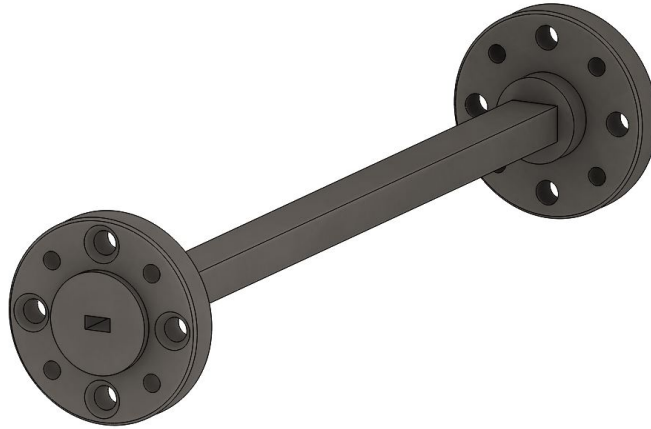
Figure 6.1: Straight 10 cm WR-10 waveguide model used for AM fabrication.
