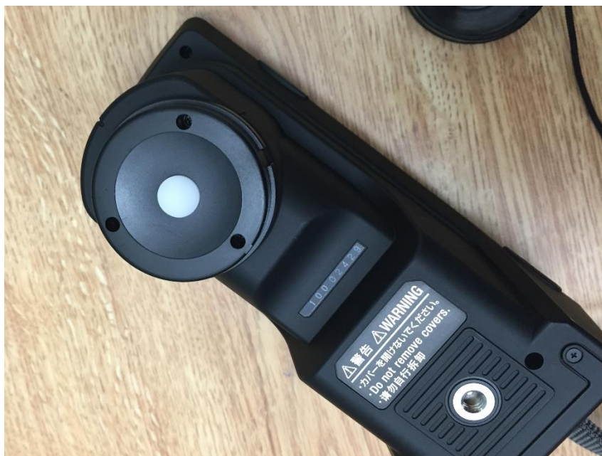
Figure 7: Konica Minolta CL-500A Illuminance Spectrophotometer
