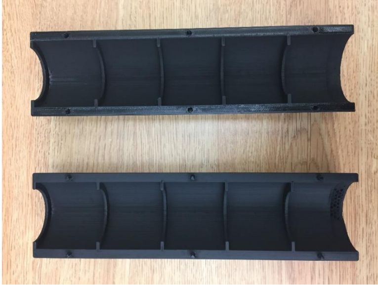
Figure 11: Spray Painted Baffle Interior
