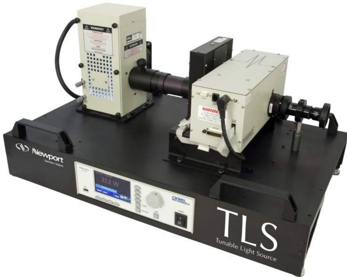
Figure 20: Monochromator with Xenon Source (41)
