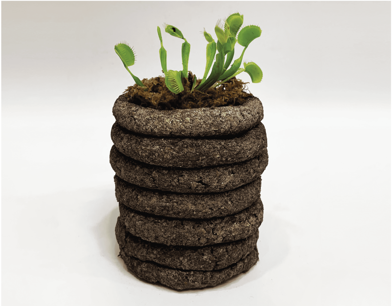
Figure 5.1: This ReClaym plant pot was one of the first artifacts I created from my food waste once I arrived at my “optimal” recipe. The pot was hand-extruded through a piping bag to create a coil pot shape. I used the pot as a home for my venus fly trap plant.
