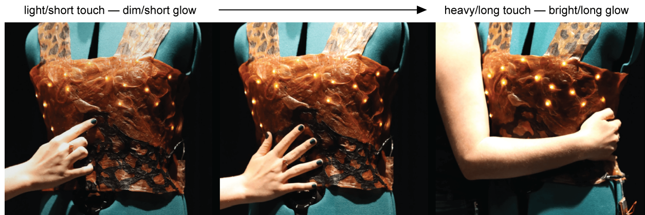
Figure 6.9: The SCOBY breastplate senses various touch interactions and displays corresponding light responses via the embedded LEDs.
