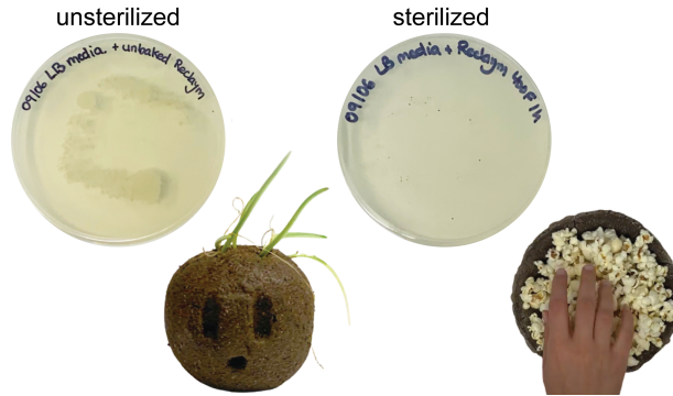
Figure 5.4: Sterility test results show the bacterial growth on LB agar plates from an unsterilized ReClaym tile and a sterilized ReClaym tile. The unsterilized ReClaym proved to work for living sculpture applications, while sterilized ReClaym was used for tableware applications.
