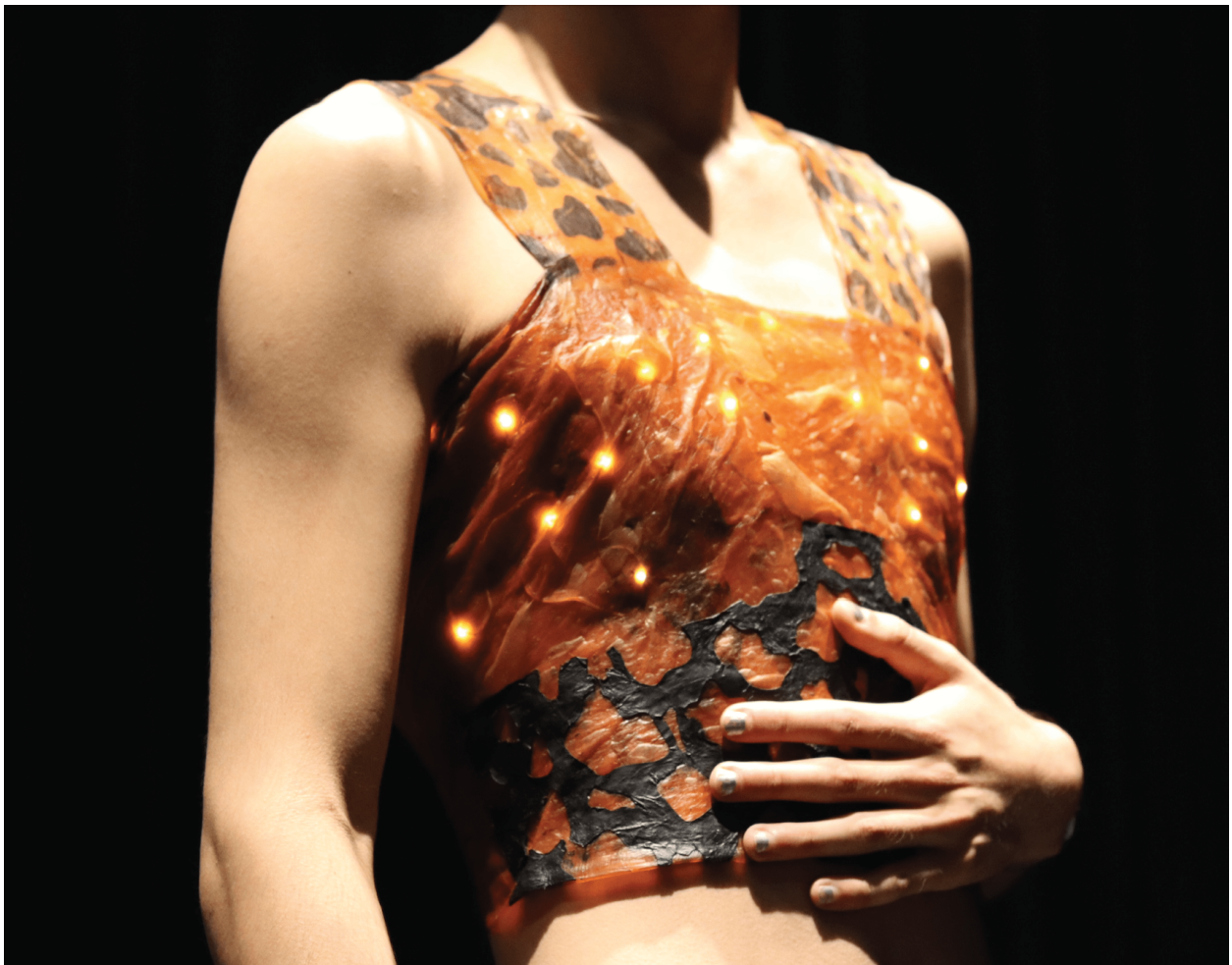
Figure 6.1: The SCOBY Breastplate is an interactive wearable created by myself, Derrek Chow, and Hyelin Choi. It is made from SCOBY and took 13 weeks to design, grow, and fabricate. When the biodegradable SCOBY touch sensor at the core of the breastplate is touched, the embedded LEDs display a corresponding light response at the top of the breastplate.
