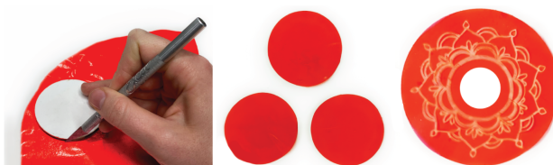
Figure 4.3: Subtractively fabricating with Alganyl by cutting it with an X-acto knife, scissors, or a laser cutter. The laser cutter was also used to engrave detailed patterns onto the surface of Alganyl.
