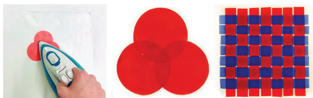
Figure 4.4: Additively fabricating with Alganyl by heat sealing pieces together with a fabric iron or the hot tip of a hot glue gun. Heat sealing can be used in conjunction with traditional textile fabrication techniques such as weaving to create composite pieces.
