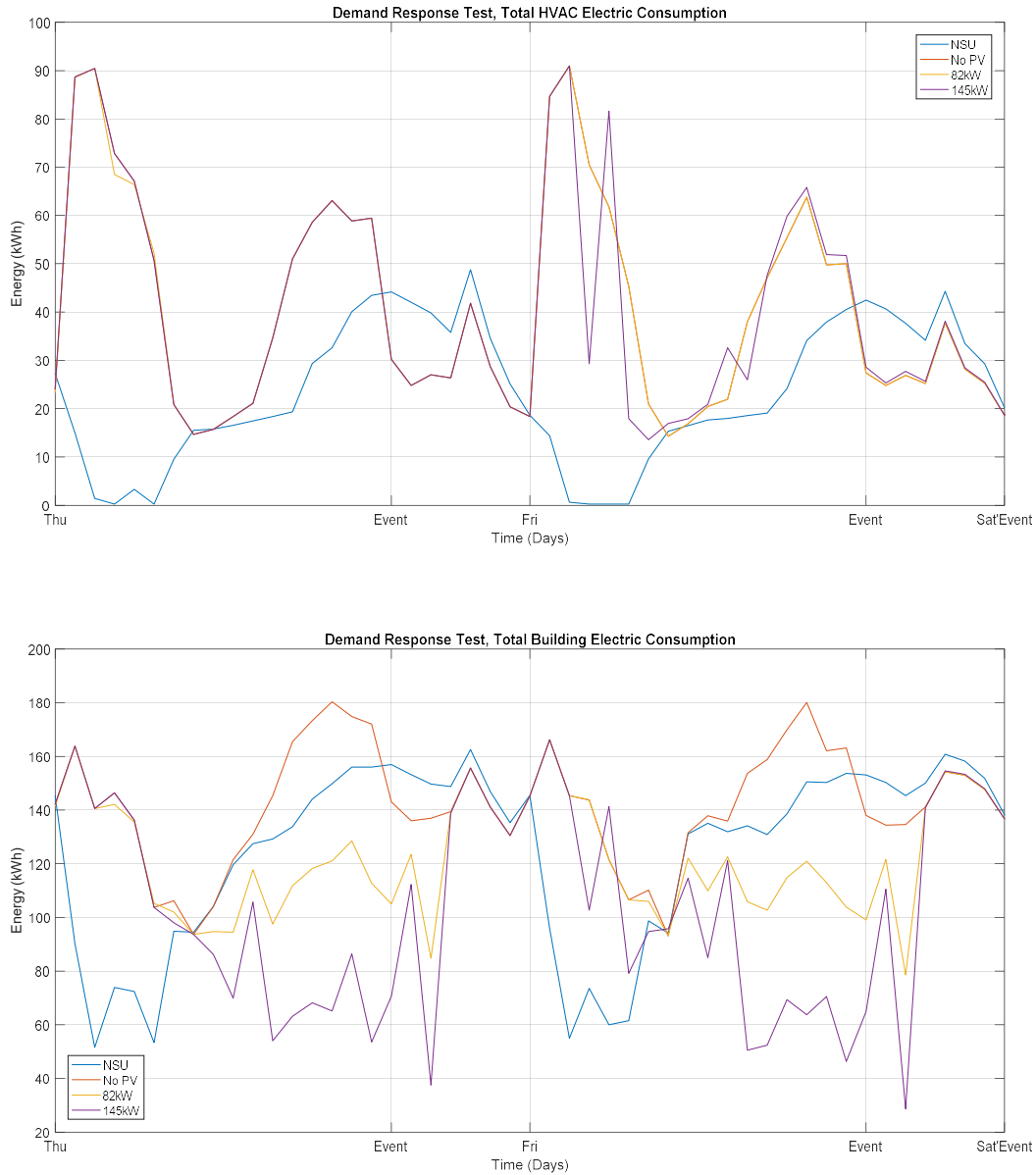
Figure 54: Demand Response Test, Total Electric Consumption
