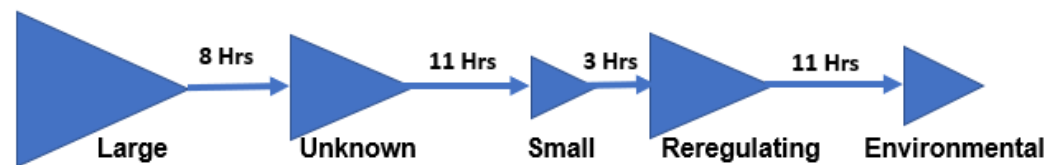
Figure 1. Schematic of the reservoirs and river reaches indicating the travel time (lags) between the reservoirs and the direction of flow.
