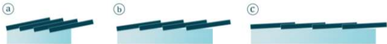
Figure 8.- Engineered scales morphology upon in plane a) compression b) unstressed c) tension
