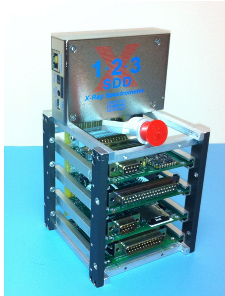
Figure 6.7: Prototype CubeSat card cage design. Figure courtesy of Tom Woods.
