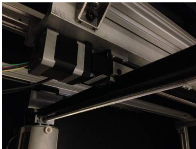
Figure 7: Rail System with Stepper Control
