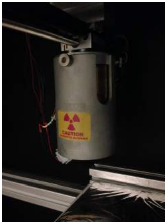
Figure 8: Strontium-90 Radiation Source
