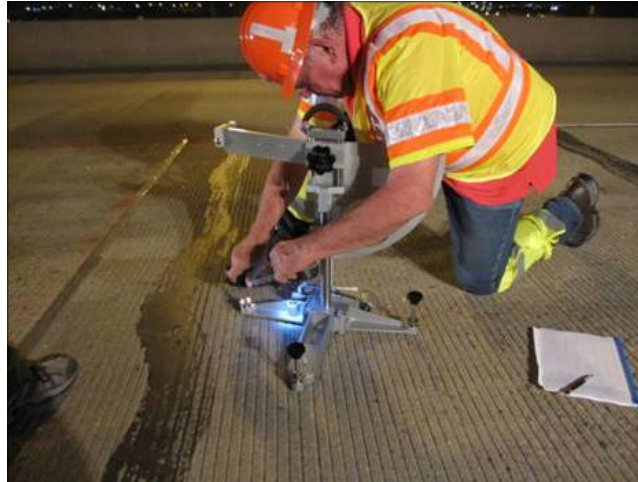
Figure 6.11 Conduction of skid resistance test
