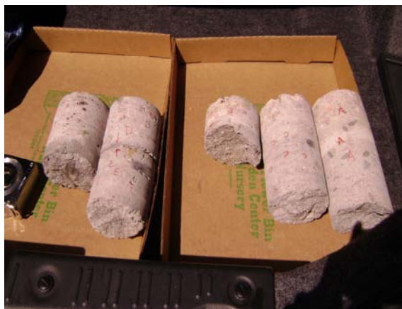
Figure 5.4 Concrete samples (Bridge G-22-BH)
