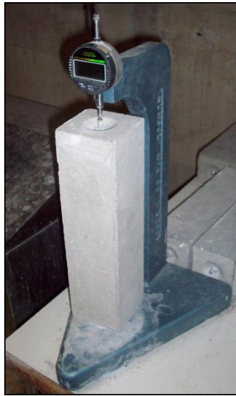
Figure 3.4 The comparator reading for length change measurement
