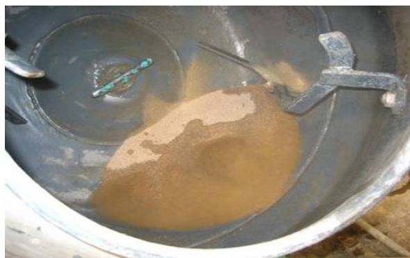
Figure 2.14 Mixing approach 2: sand enveloped mixing approach (SEMA)
