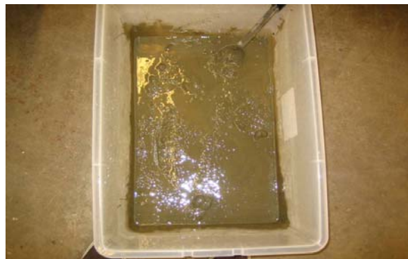
Figure 2.3 Surface treatments with cement slurry in Group 3
