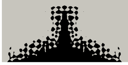
Figure 7.91: Convective design resulting from no feature size enforcement ( c_M = \infty ).
