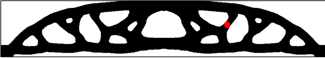
Figure 7.88: Optimized material layout for the 2D MBB beams with a minimum feature size constraint of r_x = 9h .
