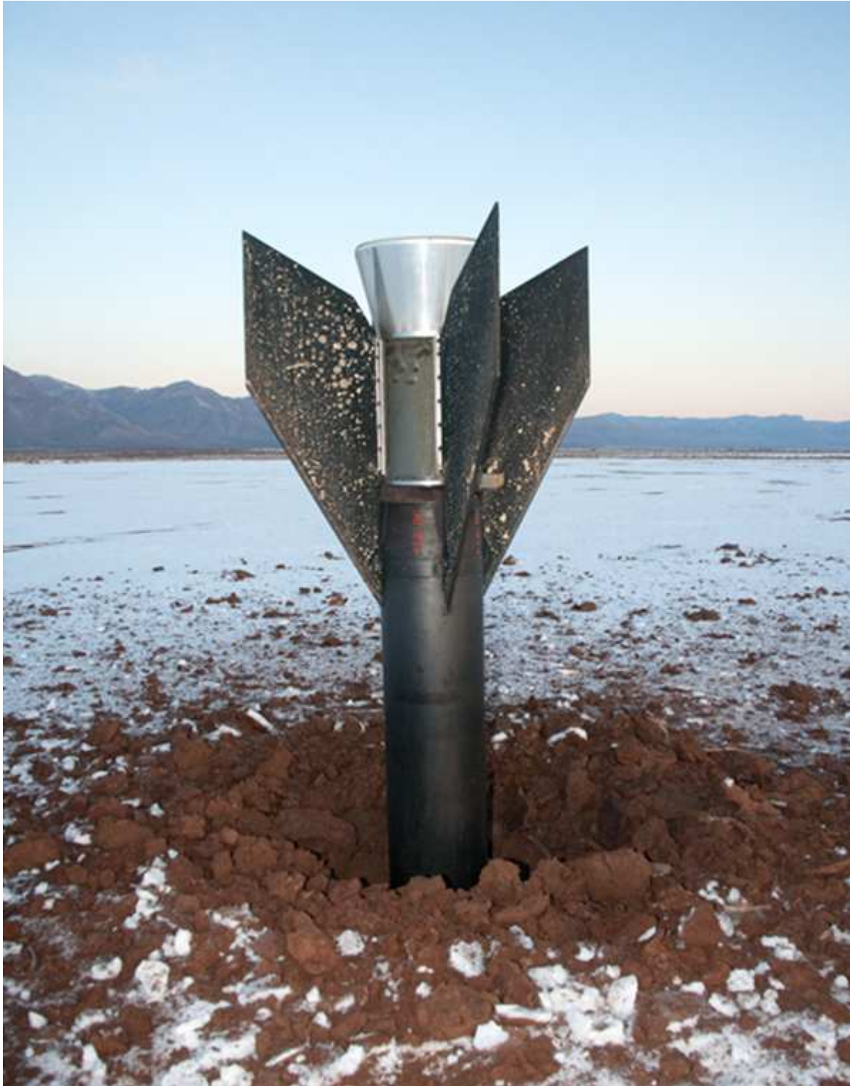
Figure 3.3 What goes up must come down, but it doesn't always look the same when it gets back. The Black Brant sustainer section is not designed to be recoverable, but it hit in soft mud and demonstrated why lawn darts are now illegal.
