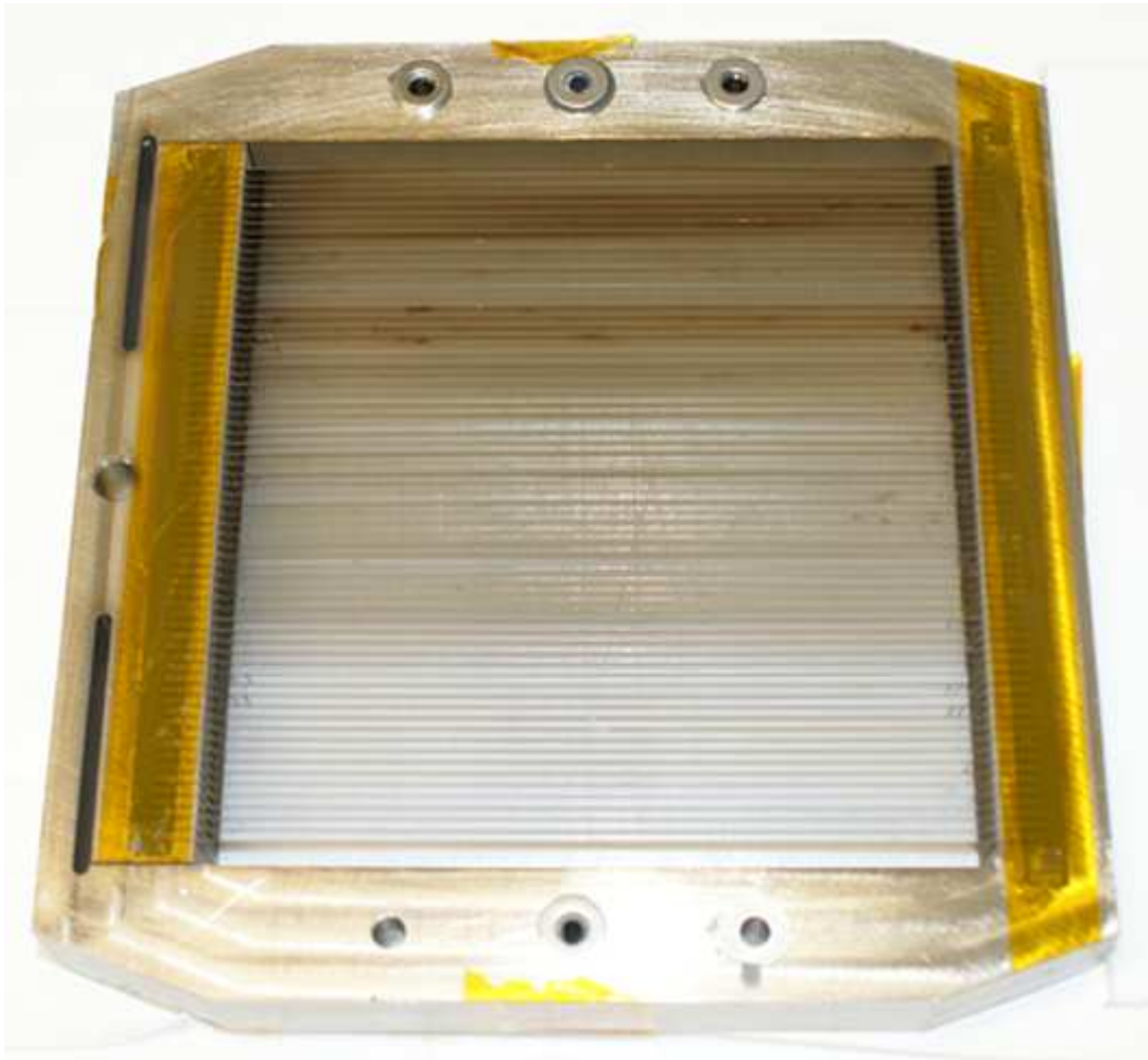
Figure 2.17 Diffraction grating array, showing the 67 off-plane mounted reflection gratings in their titanium flexure mount. The mount holds the gratings uniformly tensioned at 5 lb to reduce their deflection during launch.
