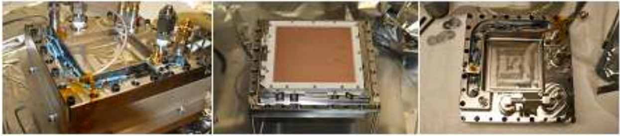
Figure 2.25 The new design of the GEM detectors, as built at the University of Iowa. Left: The fully-constructed GEM, viewed from the back. The high voltage resistor chain (blue resistors) is exposed; it was later potted in arathane for safety and durability. Middle: The interior of the GEM, revealing the GEM plates. The window and the PEEK housing, which hold the Ar/CO 2 gas, have been removed. Right: The back side of the detector, with a clearer view of the high voltage resistor chain and the gas feedthroughs.
