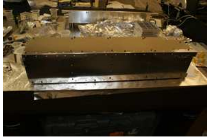
Figure 2.6 Left: Collimator stack, lacking the 12 densely-stacked plates at the top (image left) of the collimator. The five wide braces spaced at both ends and evenly in the middle carry the majority of the load between the precision-machined corner L-beams. Collimator plates slide into the slots in the corners before being fixed into place with potted sheer pins and #4-40 screws. Right: Fully assembled collimator stack, with 0.125 inch thick aluminum sheer panels affixed to the side to strengthen the tower. Light will enter at image left, and the mount to the grating bulkhead will attach at image right.
