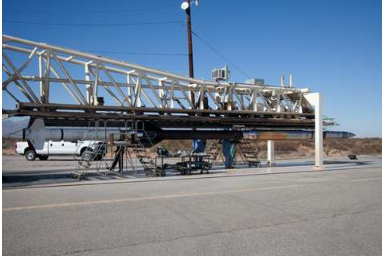
Figure 2.46 Full configuration for sounding rocket flight 36.274, carrying the CODEX payload, on the launch rail at the White Sands Missile Range. CODEX is housed in the thicker skin toward the nose of the rocket.
