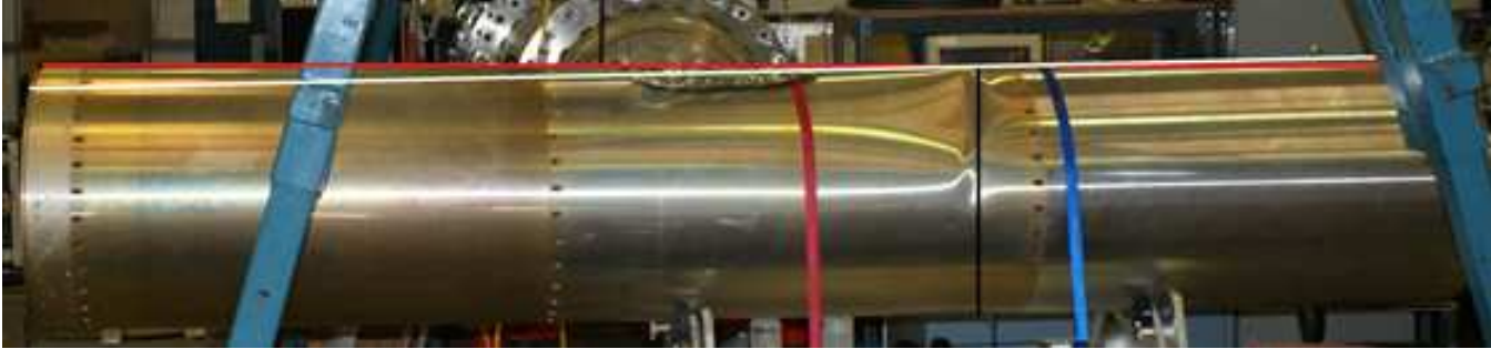
Figure 3.2 CODEX, after its return to the University of Colorado, displaying the kink it acquired on launch night. The horizontal red line is aligned with the top of the left section of the payload; the horizontal white line is aligned with the top of the right section; and the vertical black line marks the kink. The collimator and the gratings lie in the left third of the visible payload, while the optics bench comprises the right two-thirds with the detectors on the right edge of the photograph. The relative angle of the optics and the detectors — due to the kink — is 1.2^\circ , corresponding to a shift of the detectors of 4 cm perpendicular to the dispersion of the spectrograph (along the unfocused direction of the spectrum, where the spectral lines are long). The internal optics are not directly connected to the external skin, and the actual shift is under 2 cm. Due to the coarse nature of the spectrograph, however, we could not accurately measure the internal shift. For future payloads, a mirror placed on the detector bulkhead would have allowed for such a measurement using a theodolite. There is no good explanation of the cause of the kink.
