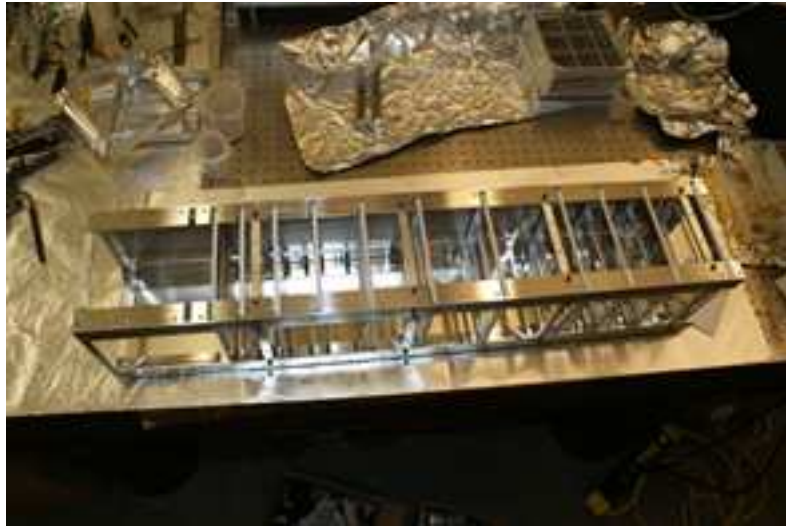
Figure 2.6 Left: Collimator stack, lacking the 12 densely-stacked plates at the top (image left) of the collimator. The five wide braces spaced at both ends and evenly in the middle carry the majority of the load between the precision-machined corner L-beams. Collimator plates slide into the slots in the corners before being fixed into place with potted sheer pins and #4-40 screws. Right: Fully assembled collimator stack, with 0.125 inch thick aluminum sheer panels affixed to the side to strengthen the tower. Light will enter at image left, and the mount to the grating bulkhead will attach at image right.
