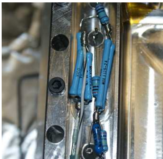
Figure 2.26 Part of the high voltage resistor chain, carrying -4,000 V at its start, in the new GEM detectors built for CODEX. The close-packing of the resistors was ameliorated by an arathane insulator potting the channel around the detectors to prevent arcing.
