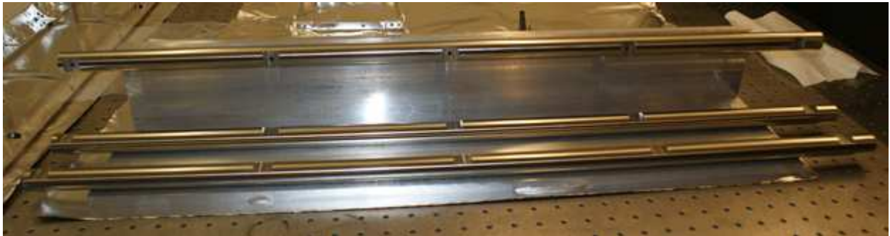
Figure 2.5 Alignment fixture showing the two bars that provided the y alignment edge along the bottom and the x alignment edge along the side. The two bars along the y edge defined the plate rotation such that, between the three plates and the corners of the collimator structure, every plate position was fully defined. The fixture was flat to within 38\text{ }\mu\text{m} (measured as 0.0015 inches) relative to a flat granite table, and alignment of plates to the fixture could be done to 25\text{ }\mu\text{m} (0.001 inches).
