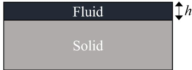
**Figure 3-1.** Schematic of the model used to study guided wave propagation at the interface between a liquid layer of finite thickness  $h$  and a solid.
