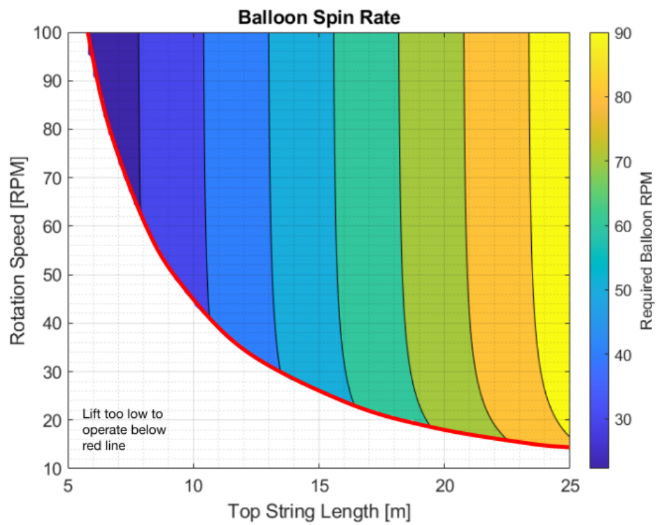
Figure 5.8: Effects of various string lengths and rotation speeds on balloon spin rate. 3.6 m balloon (at ground level) for a 1 m/s translation at 30 km.
