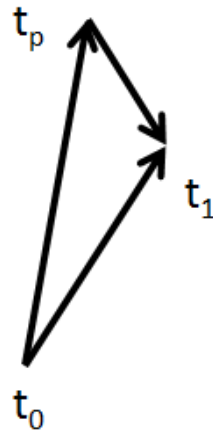
Figure 3.1: Ship Drift Triangle
