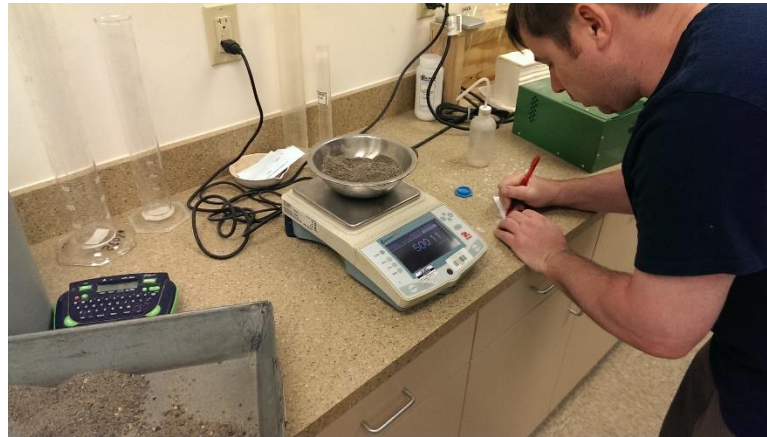
Figure 66 - A 500g sample of fine aggregate at SSD is weighed
