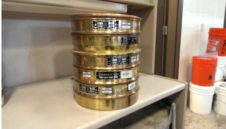
Figure 72 Sieve stack ready for coarse aggregate analysis
