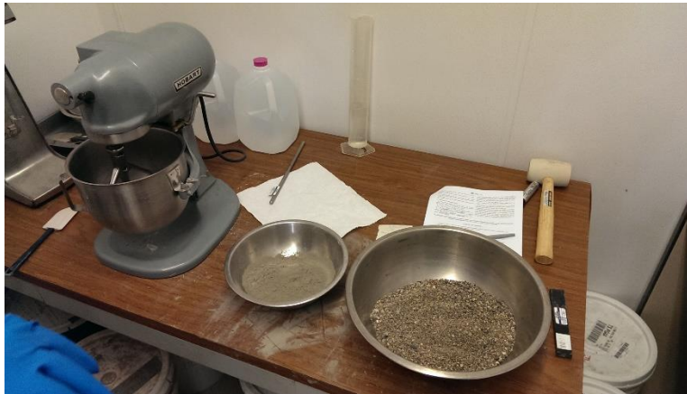
Figure 46 – Mixer with measured cement, water, and aggregate
