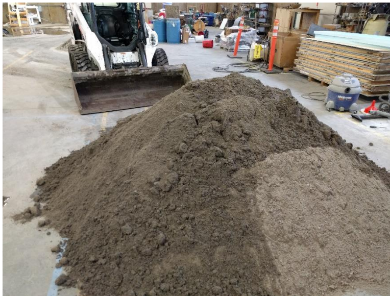
Figure 31 - Mixing fine aggregate and forming into pile.
