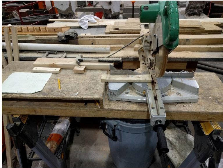
Figure 19 - Cutting wooden blocks for the welding jig.
