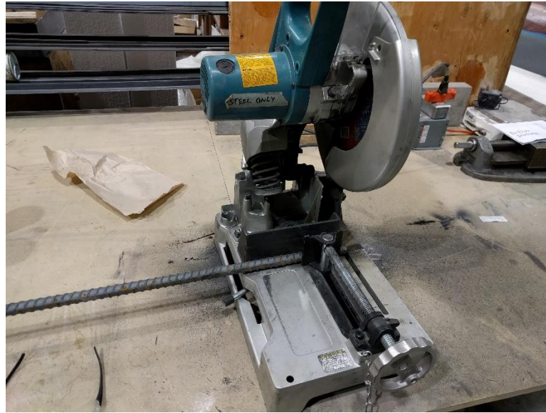
Figure 22 - Cutting reinforcing bar
