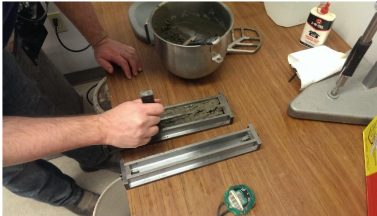
Figure 48 - Tamping mortar into molds
