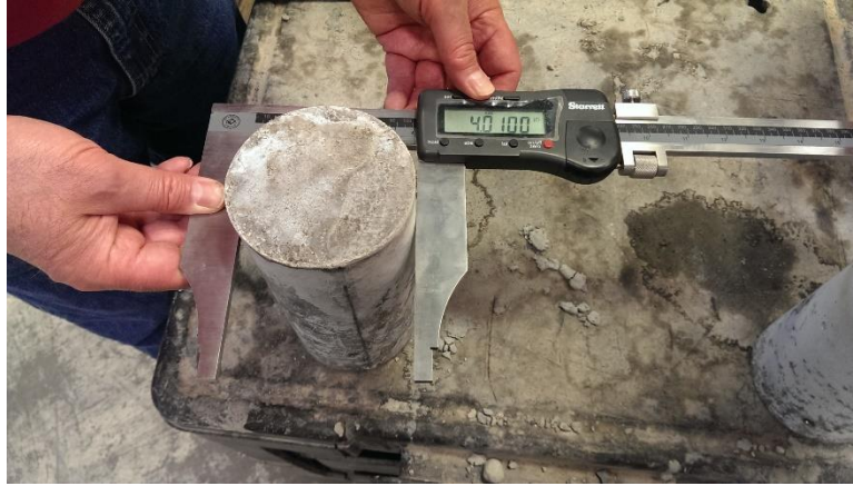
Figure 90 - Measuring cylinder diameter
