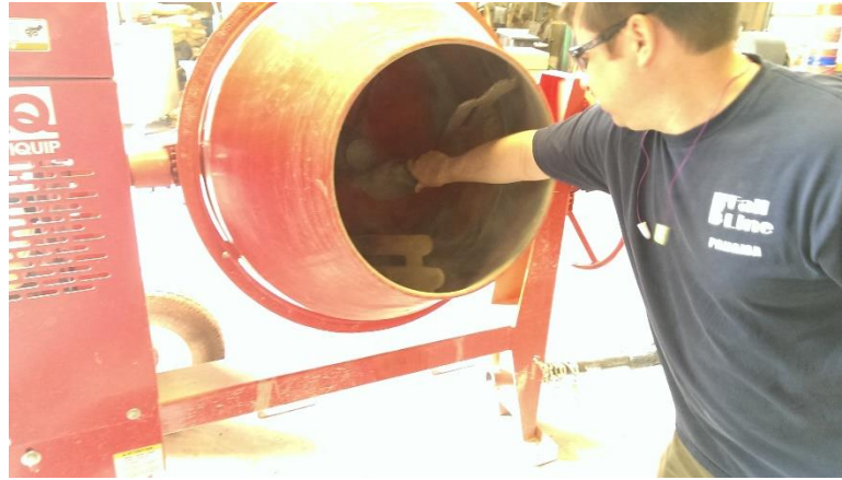
Figure 74 - Buttering the mixer
