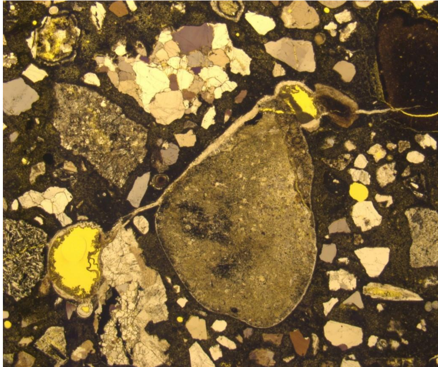
Figure 5: Mortar-bar with crushed coarse aggregate – the same area as in Figure 4. Plane polarized light.
