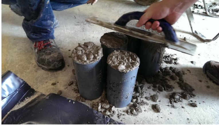
Figure 88 - Striking off cylinder molds
