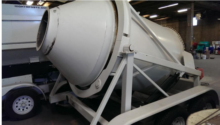
Figure 28 - The three-cubic yard mixer at Fall Line
