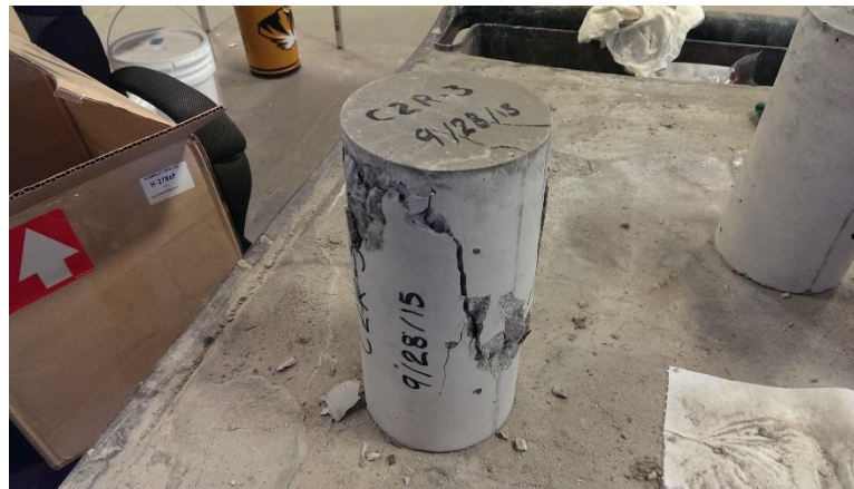
Figure 93 - Fractured cylinder after testing
