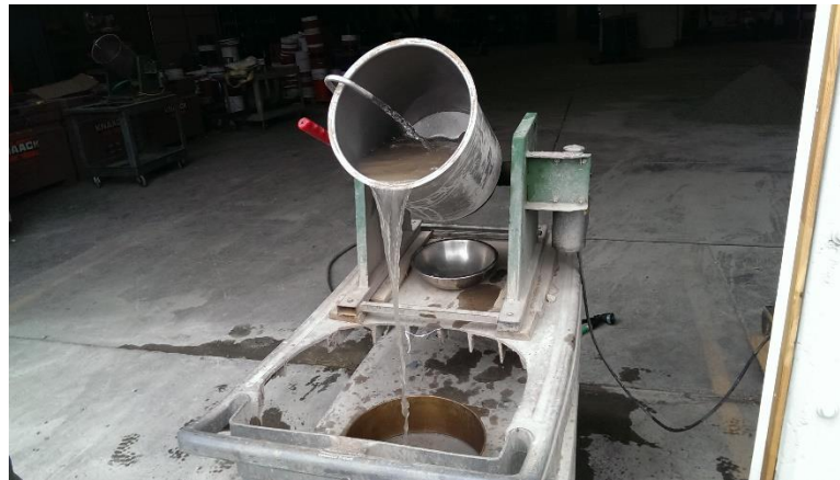
Figure 71- Washing aggregate in preparation for sieve analysis
