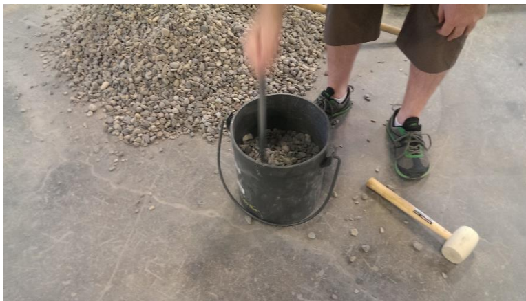
Figure 70 - Each lift is rodded 25 times.
