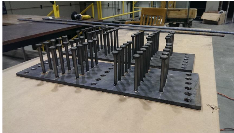
Figure 8 - Sample end plates with shear studs
