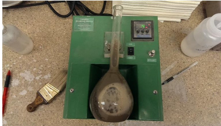
Figure 68 - The volumetric flask is rotated to remove trapped air.
