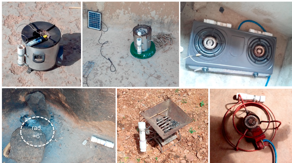
Fig. 1. Stove usage monitors (SUMs), comprised of thermocouple dataloggers (SSN-61) enclosed in PVC piping (2-inch diameter, 9-inch length), installed on 6 varieties of stove types encountered in the Prices, Peers and Perceptions (P3) cookstove study. Clockwise from the top left; Greenway Jumbo rocket stove (thermocouple logger visible), ACE1 semi-gasifier stove, 2-burner LPG stove, locally made 1-burner LPG stove, locally made charcoal-burning ‘coalpot’ and the traditional three stone fire (TSF) with standard placement of probe terminus 6 inches from center of combustion area. Additional instrumentation images can be found in SI Section 1 ).
