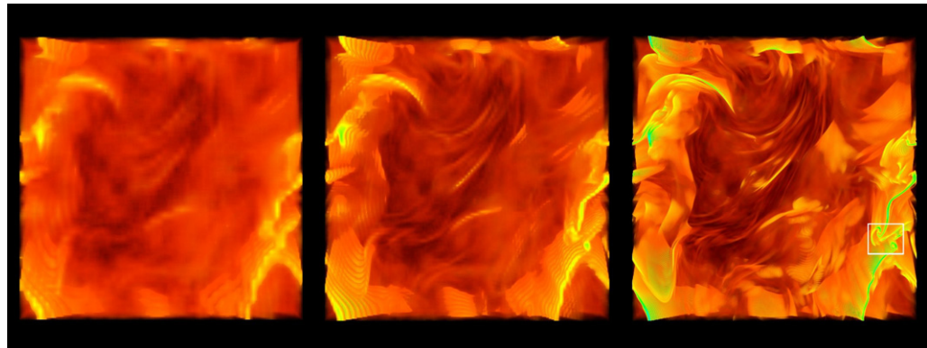
Figure 10. 3D rendering of current density intensity in a slice of 1536 \times 1536 \times 150 grid points. From left to right, visualizations at 1/32 , 1/16 and 1/4 of the total resolution are shown. The white box in the right indicates a small subregion where rolling of current sheets is observed.
