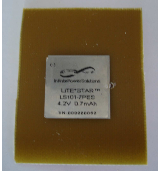
Figure 7.5: Photo of a 2.8 GHz patch antenna made from a battery and 60 mil FR4 substrate. Battery dimensions are 25 mm \times 25 mm.
