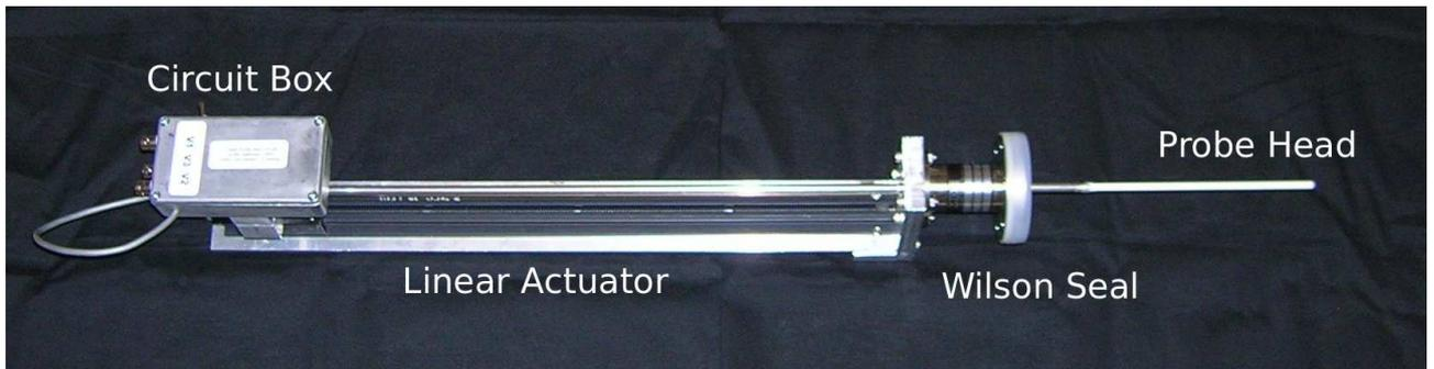
Figure 3.12: Photograph of the triple probe assembly.
