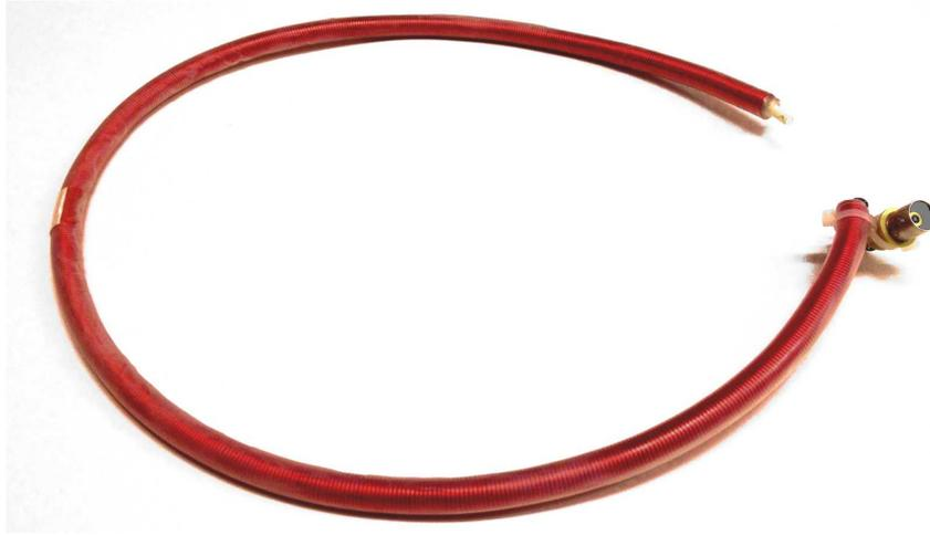
Figure 3.8: Photograph of a Rogowski coil built for measuring the plasma gun current.
