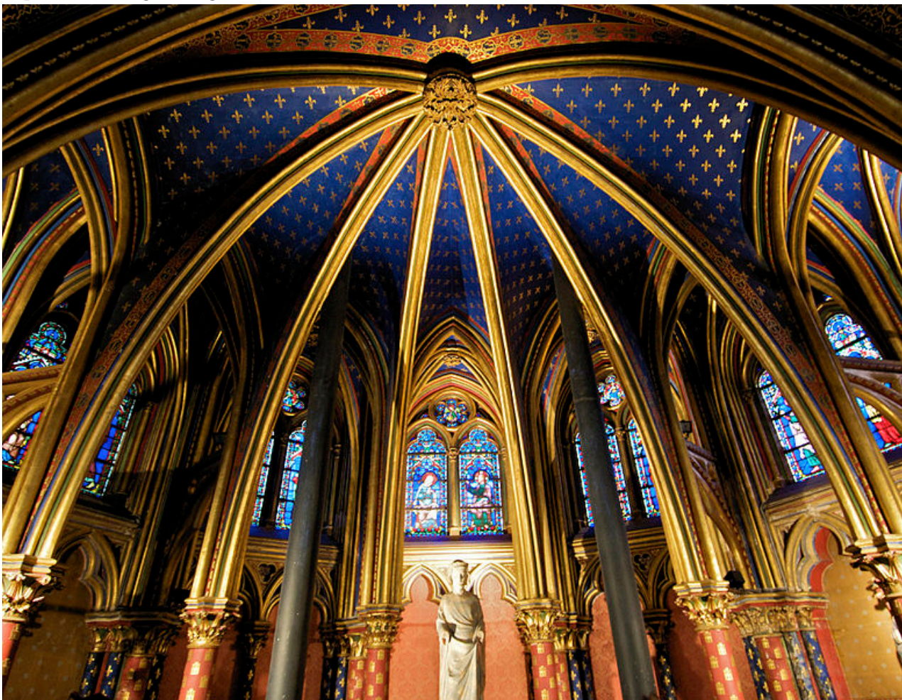
St. Chapelle exhibits the classic features of Gothic architecture: pointed arches over the windows, large stained glass windows, and webbed vaulting on impressively high ceilings.
