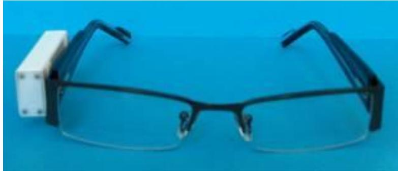
**Figure 2: The OT LightWatcher data recorder attached to an eyeglasses frame.** The OT LightWatcher data recorder measures eye-level light exposure in the red (620 nm), green (540 nm), and blue (465 nm) bands every 10 seconds.
