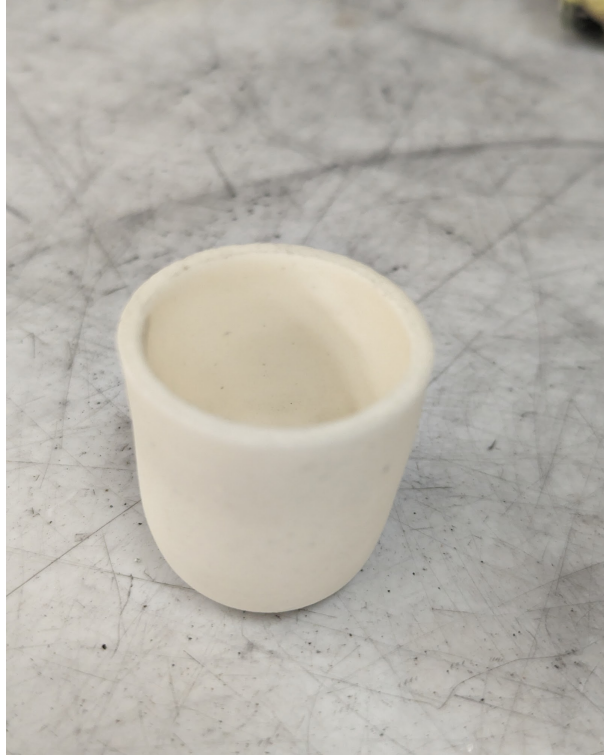
Figure 12: Alumina crucible used for flux growth
