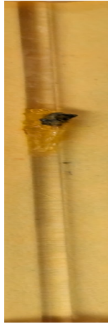
Figure 9: Quartz rod with attached sample
