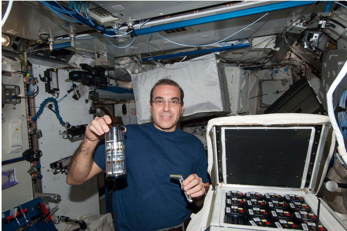
FIGURE 1 | NASA Astronaut Rick Mastracchio shown holding a GAP in his right hand and the crank used to perform an activation in the other as he performed the experimental operations onboard the International Space Station. The open CGBA incubator loaded with other 15 GAPs is in the bottom right. Image: NASA. The individual in this manuscript has given written informed consent to publish this image.
